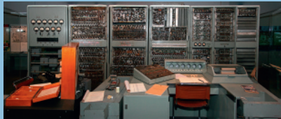
TL.1.7 The first stored-program computer constructed in Australia used a mercury line memory and could generate music.
