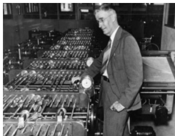
Fig. 1.3 Vannevar Bush's Differential Analyzer was a complicated analog computer that used rotating discs and wheels for computing integrals. The complete machine occupied a room and linked several integration units connected by metal rods and gears. The Differential Analyzer was used to solve ordinary differential equations to calculate the trajectories of shells at the U.S. Army Ballistics Research Laboratory in Aberdeen, Maryland.
