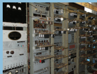
TL.1.3. The first stored program computer. The memory was constructed from Cathode Ray Tubes.
