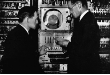
Fig. 1.14 Tom Kilburn and Freddie Williams with the “Baby” computer in Manchester. The machine had only seven instructions and had 32 \times 32 bits of main memory implemented using a cathode ray tube.
