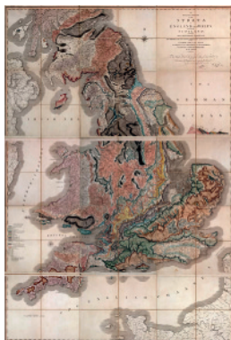
Fig. 1.1 The famous geological map of Great Britain devised by William “Strata” Smith (1769–1839). Smith was a canal and mining engineer who had observed the systematic layering of rocks in the mines. In 1815, he published the “map that changed the world” – the first large-scale geological map of Britain. Smith was first to formulate the superposition principle by which rocks are successively laid down on older layers. It is a similar layer-by-layer approach in computer science that allows us to design complex systems with hundreds of millions of components.
