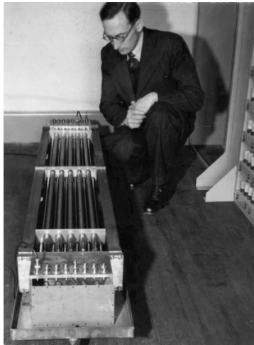
B.2.6. Maurice Wilkes (1913–2010) seen here checking a mercury delay-line memory. He was a major figure in the history of British computing and at the University of Cambridge he led the team that designed and built the first fully operational stored-program computer.
