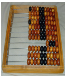
Fig. 2.6. A Russian abacus, used in almost all shops across the Soviet Union well into the 1990s. It is fast, reliable, and requires no electricity or batteries. It was common practice in shops that the results calculated by an electronic till were double-checked on the abacus.
