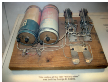
Fig. 2.15. The first binary adder, consisting of two battery cells, wires, two telephone relays, two light bulbs, pieces of wire, and a switch made from a tobacco tin.
