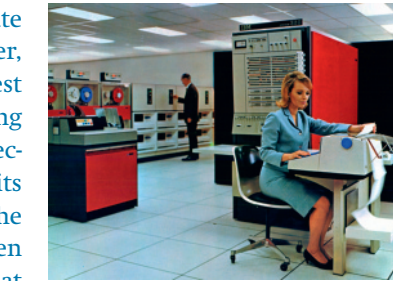
Fig. 3.15. The IBM System/360 was a family of general-purpose mainframe computers delivered in 1965. It was the first line of computers designed to be compatible with one another.
