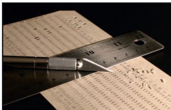
Fig. 3.1. Carving holes on a punch card. The software in the early days of computing was represented by these holes but the cards were actually punched by machines.
