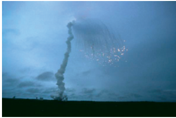
Fig. 4.15. Photo of the destruction of the first launch of the Ariane 5 Flight 501 rocket. Just thirty-seven seconds into the launch, the trajectory suddenly tilted by almost 90 degrees and the rocket self-destructed. The software error occurred during data conversion from a 64-bit floating-point number to a 16-bit signed integer. This led to a sequence of events that resulted in a complete loss of the guidance system.
