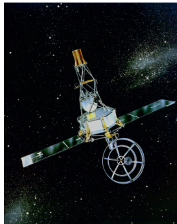
Fig. 4.14. Mariner 1 Space probe to Venus was the first interplanetary mission aiming to put a satellite around Venus. There are various stories about the reason why this mission had to be aborted. Most of them firmly point at a bug in the FORTRAN code of the guidance system that unexpectedly changed the trajectory of the rocket. A hyphen (overbar) missed in a mathematical expression led to the $80 million failure. Five months later the Mariner 2 was successfully launched and completed the mission.
