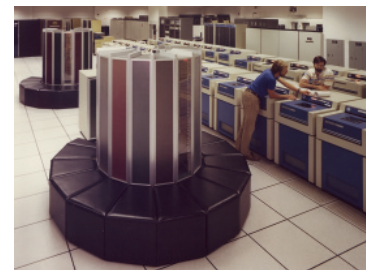
Fig. 7.23. A photograph of two Cray-1 supercomputers at Lawrence Livermore National Laboratory. The upholstered bench around the computing tower hides the power supply and the intricate network of Freon cooling pipes. The supercomputer was sometimes referred to as “the most expensive seat in the world.”
