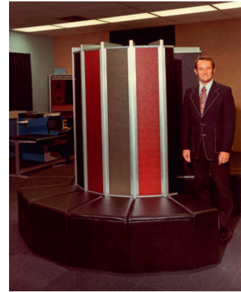
B.7.12. The name of Seymour Cray (1925–96) has become inseparable from supercomputers. Cray was one of the first to recognize that maximizing the speed of moving data between the processor and memory and hiding memory latency using a vector pipeline was the key to achieving high-performance computing speeds. He is pictured here next to a Cray-1 supercomputer.
