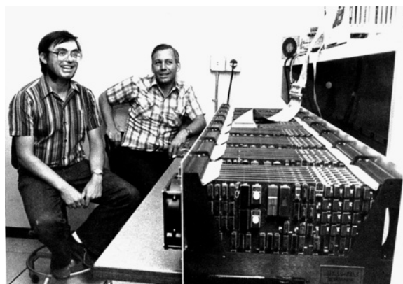
Fig. 7.24. Geoffrey Fox and Chuck Seitz pictured next to the Caltech Cosmic Cube machine. This parallel computer became operational in October 1983 and contained sixty-four nodes each with 128 kilobyte memory. A computing node was made up from an Intel 8086 processor with an 8087 coprocessor for fast floating-point operations. The nodes were linked together in a so-called hypercube topology – several cubes connected together – for minimizing communication delays between nodes. The size of the computer was only six cubic feet and drew less than a kilowatt of power. The Cosmic Cube and its successors represented a serious challenge for the Cray vector supercomputers. Today all the highest-performing machines use a distributed memory message-passing architecture similar to the Caltech design.
