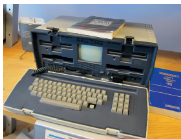
Fig. 8.25. The first "Portable Computer" – the Osborne 1 – was released in 1981. It weighed 24.5 pounds (12 kg) and cost US$1795 – just more than half the cost of a computer from other manufacturers with comparable features – and ran the CP/M operating system. It was designed to fit under an airline seat. At its peak, the Osborne Computer Corporation was shipping ten thousand units per month.
