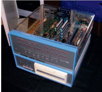
Fig. 8.5. The MITS Altair 8800. Most do-it-yourself hobbyists did not want to have to buy all the integrated circuits and other components needed to build the computer. The appeal of the Altair 8800 was that it was the first build-your-own-computer kit.
