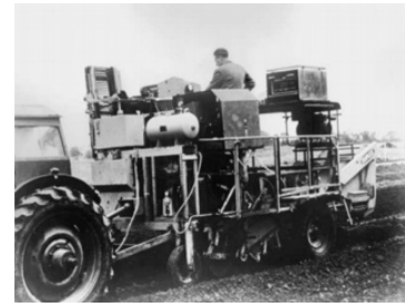
Fig. 8.22. A PDP-8 on a tractor used for controlling sowing.
