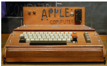
Fig. 8.9. Steve Wozniak demonstrated the prototype Apple I at the Homebrew Computer Club in 1976. For $666.66, buyers received a blank printed circuit board, a parts kit, and sixteen-page assembly manual. The power supply, keyboard, storage system, and display were not included.
