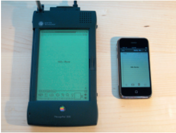
Fig. 8.18. The first “Newton” message pad from Apple was released in 1993. This handheld device used an ARM RISC processor and ran various applications for handwriting recognition, note taking, sketching, Internet access, and other productivity tools. The more sophisticated iPhone incorporates many features of its predecessor.
