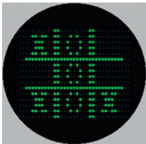
Fig. 9.1. Alexander (Sandy) Douglas created a version of tic-tac-toe or noughts and crosses for the Cambridge EDSAC computer in 1952. The output was displayed on a CRT screen.
