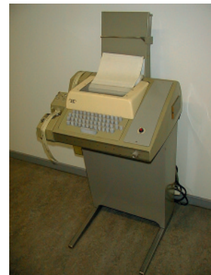
Fig. 9.18. The photograph shows the Teletype Corporation’s Model-33 terminal also known as an ASR-33 (ASR stands for Automatic Send Receive). The model was introduced in 1963 and more than half a million teletypes had been produced by 1975. The 500000th machine was plated with gold and exhibited.
