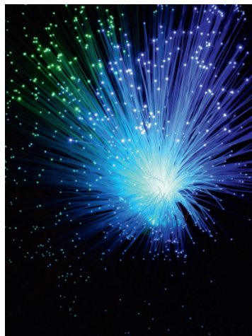
Fig. 10.23. Light conducted by a bundle of optical fibers. The core of the fiber is only a few microns wide. A typical human hair is about fifty microns wide, so optical fibers are about a tenth of the diameter of hair.
