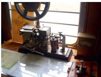
Fig. 10.1. An advanced version of a telegraph with a printing receiver and transmitter.
