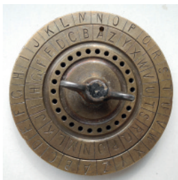
Fig. 12.11. Cipher disk invented by the Renaissance artist Leon Battista Alberti (1404–72). The brass inner disk can be rotated to align its letters with the letters of the outer circle.
