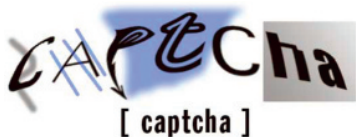
Fig. 13.3. CAPTCHAs can be easily read by a human, but not by a computer. This is one commonly used mechanism to distinguish between human visitors to websites and robotic crawlers.
