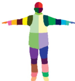
Fig. 14.6. Color-coded pattern of thirty-one different body parts used by the body pose algorithm developed by Microsoft researchers for the Kinect Xbox application.
