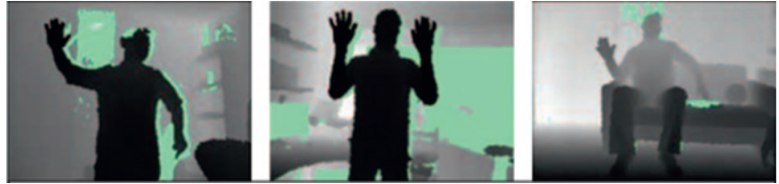
Fig. 14.5. Some example images from the Kinect camera. Nearby points are dark gray, and farther points are light gray. In the green areas, no infrared data was captured.
