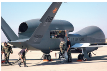
Fig. 16.7. The Northrop Grumman Global Hawk drone can fly at sixty thousand feet for flights as long as thirty hours.
