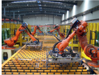
Fig. 16.2. Robots handling the delicate operation of glass panel unloading.
