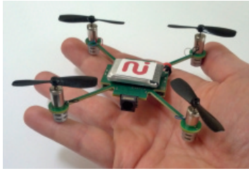
Fig. 16.8. The McCam quadcopter is a miniature drone that can follow and photograph you wherever you go and then upload the video images to your smart phone.
