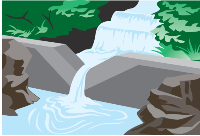
Figure 5.3 All of the water that drains from the Hubbard Brook watershed flows past a dam like this one. The V-shaped notch makes it easier for scientists to take samples and measure the rate of water flow.
