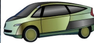
The yellow box fish provided a design model for the car shown here. The fish is the result of millions of years of natural selection for two traits that are also important in cars: efficient aerodynamics and maximum interior space.
