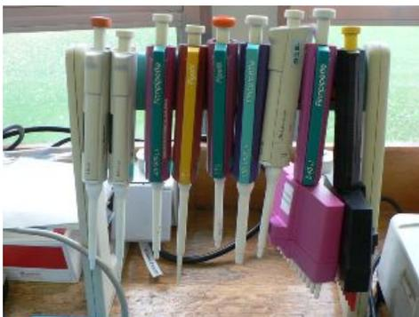
Figure 1.29: Pipettes are small, but important tools in many biology labs. Micropipettes, such as these here, are calibrated to measure very small amounts of liquids. For example, 100 microliters (100  $\mu\text{L}$ ) which is about half the volume of your little finger tip; or even 1  $\mu\text{L}$ , which is smaller than a drop of water. (16)
