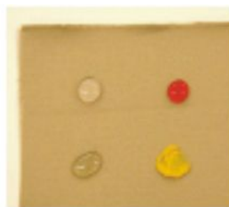
Nano-Care fabrics with water, cranberry juice, vegetable oil, and mustard after 30 minutes (left) and wiped off with wet paper towel (right)
