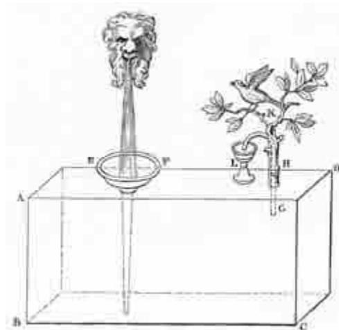
The flow of water into a sealed container forces air out through a small bent tube. The air, bubbling into a cup of water, sounds like a bird singing. (The Pneumatics of Hero of Alexandria, page
