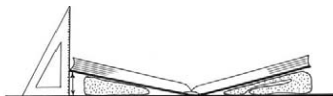
Fig. 6-29 To leave both hands free for measuring, place temporary supports under the book covers
