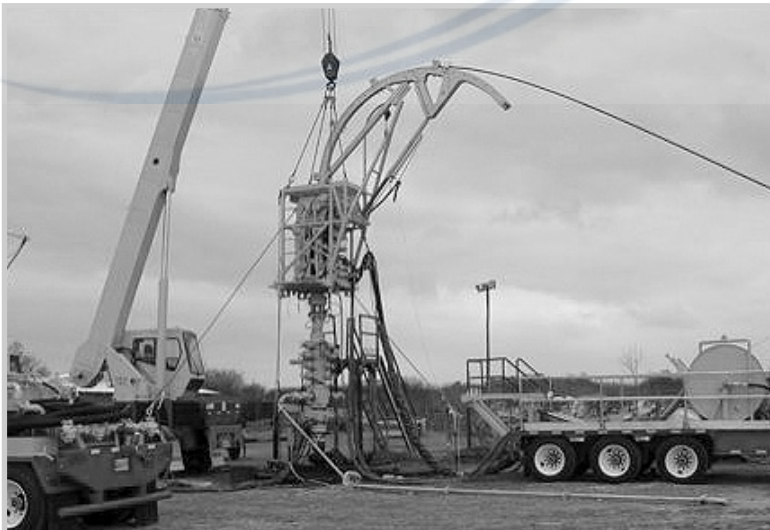
Fig. 10-3. CT operation. Flexible tubing is taken from the reel and “injected” into the well through its existing production string. The power for the injection process is supplied by the hydraulic lines that extend from the trailer to the platform on the right of the photo. Note the series of blowout preventers stacked on top of the christmas tree (the assembly with the wheel controlled valves). Courtesy of BJ Coiltech
