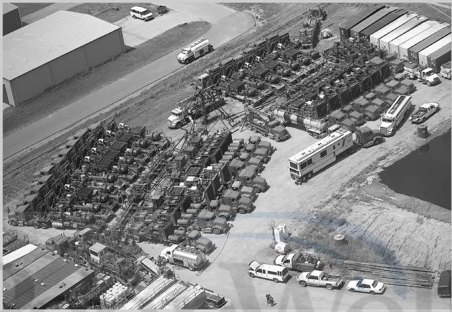
Fig. 10–6. Well site with truck-mounted pumps tied together. In this way, high pressure can be obtained to create a large fracture in target formation.
