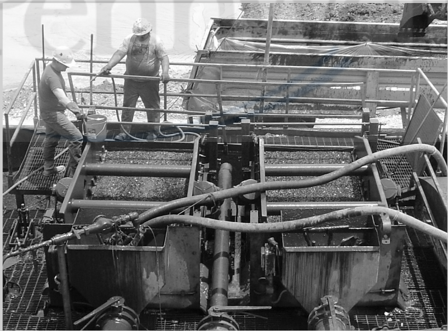
Fig. 5–15. Shale shakers. Drilling fluid carrying rock debris is circulated across vibrating screens. This separates the chips from the liquid mud, allowing its reuse. Samples of the chips (known as “cuttings”) maybe collected from the shakers. Courtesy of Bill Booker.
