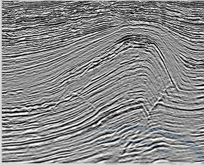
Fig. 2–22. 2D seismic display of an anticlinal feature (refer to color plate for hydrocarbon indicators shown in red). Courtesy Landmark Graphics.
