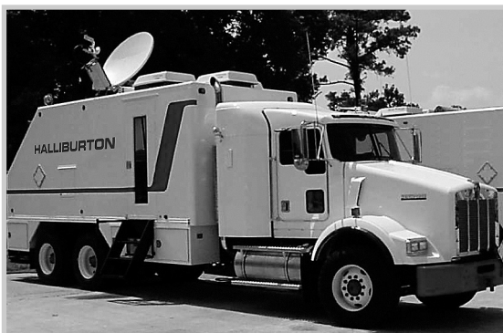
Fig. 6–9. Logging truck. The vehicle transports all the necessary equipment and houses the computerized recording devices.
