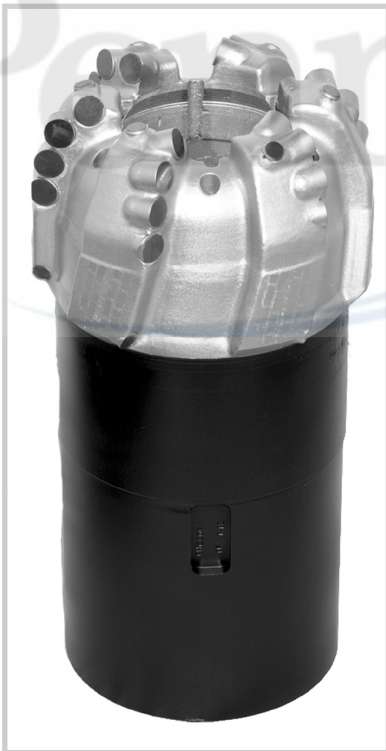
Fig. 6–12. Coring bit. The bit cuts a cylindrical column of rock that passes up the center of the bit and into a section of special pipe above the bit called a “core barrel.”
