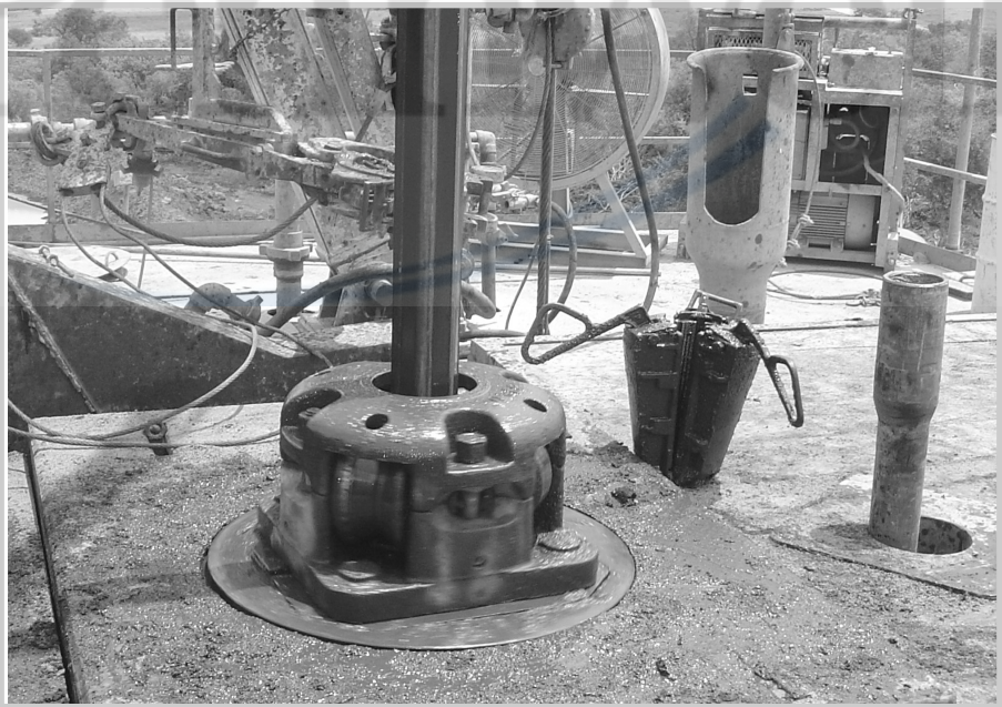
Fig. 5–8. Rotary table, kelly, and kelly bushing. The rotary table is the round element into which the kelly bushing fits. Through the bushing slides the forty-foot long kelly. In the right background is a set of slips and the top end of a joint of drill pipe, sitting in the “mousehole.” Behind the slips is the “rathole” where the kelly is set aside during the connection of the next joint of drill pipe.
