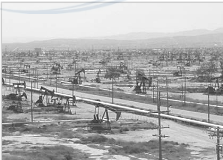
Fig. 8–17. Pump jacks in a steam drive project. The Bellridge Field, California. Courtesy of Aera Energy.
