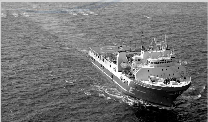
Fig. 2–20. Seismic vessel. The wake far behind the vessel is formed by the hydrophone streamers being towed. Courtesy of Veritas DGC.
