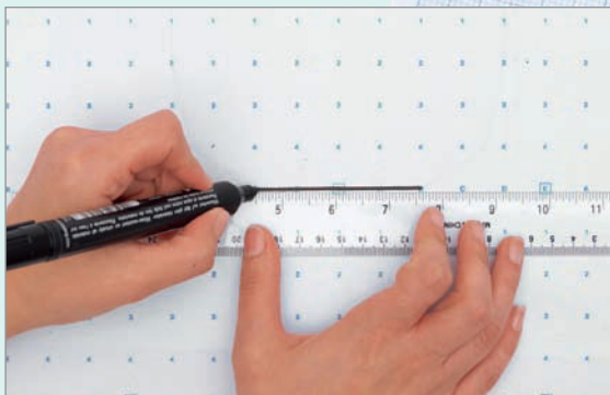
The marks on spot-and-cross paper can be used as guides for the lines of the garment shape you're drawing.
