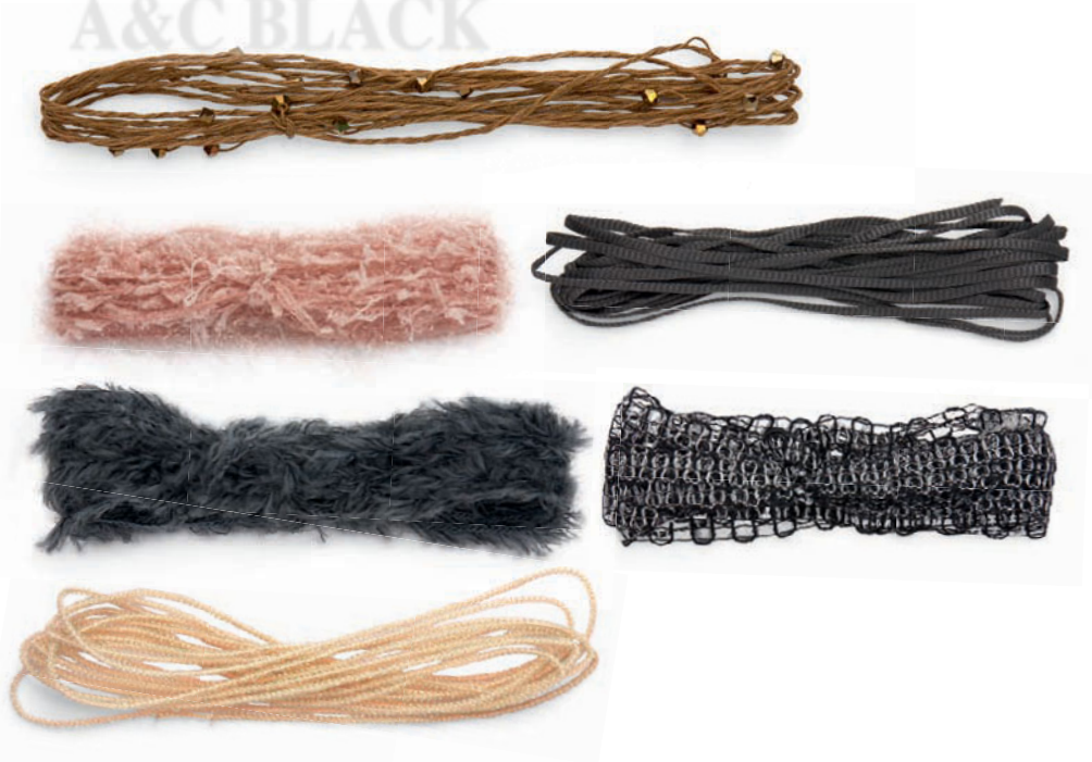
Fancy yarns shown here, clockwise from the top: Cotton twist with beads; viscose ribbon yarn; textured ribbon yarn; Lurex corded yarn; synthetic-mix mohair; feather yarn spun with man-made fibres and paper.
