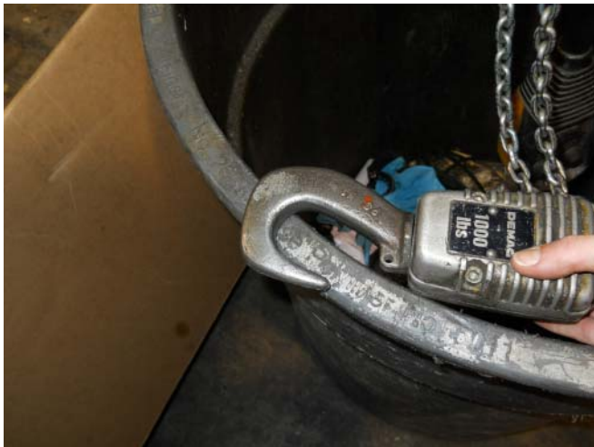
Figure 14.2. Hoist with a missing safety latch.
