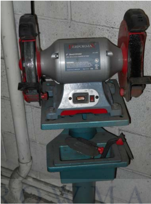
Figure 3.1. Bench grinder missing machine guards.
