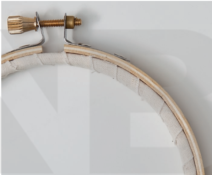
I wrap the inner ring with a ¾"-wide strip of unbleached muslin.
