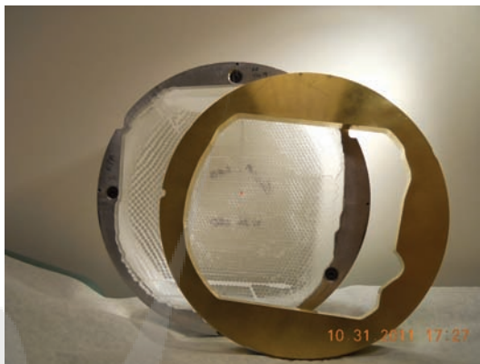
FIGURE 1 Patient specific brass aperture and Lucite™ compensator for chest wall treatment following mastectomy. The brass aperture allows for shaping of the field in the beam’s eye view (similar to the use of multileaf collimator or cerrobend blocks used for photons). The Lucite™ compensator allows for distal shaping of the proton beam and accounts for heterogeneity of the tissue in the path of the beam.
