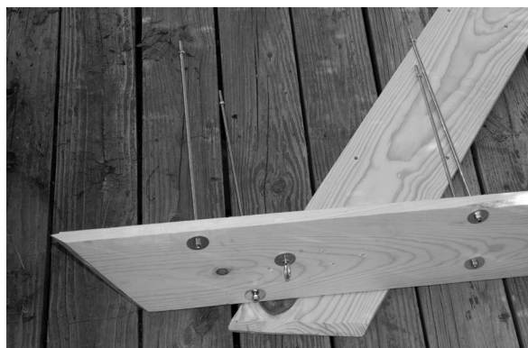
Here the four threaded rods (here 18 inches long) have been added to the one side of the planer, with fender washers on each side of the nuts to prevent pull-through and wear when fishing.
