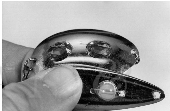
The finished lure with the bead in place and wired to the spoon blank. A simpler way to get a similar effect is shown in the top spoon—using plastic craft “jewels” glued to the blade.
