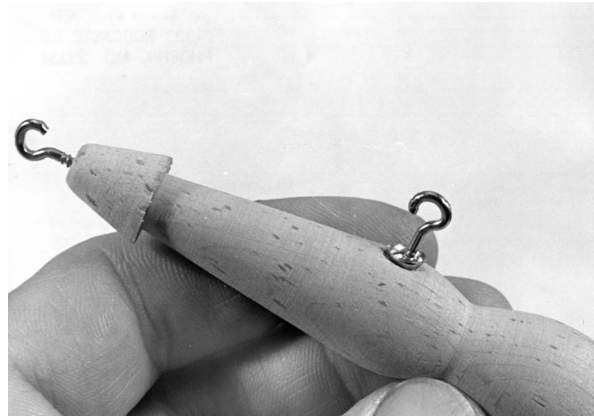
Open screw eyes in the plug body to check for position before painting and assembling. The belly screw eye uses a cup washer, fitted into a hole countersunk into the wood body.
