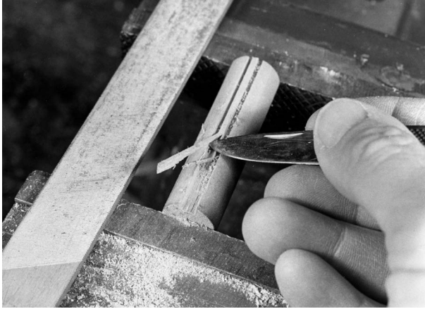
Making a bubbler for a lure by cutting four grooves around the perimeter of a dowel for passage of air and water through the lure.
