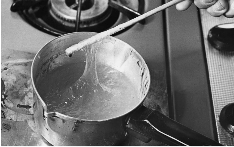
To prevent burning and smells, use low heat to melt the plastic. The plastic will first turn thick and lumpy—like tapioca—then turn thin, clear, and smooth. Shown is the “tapioca” stage.
