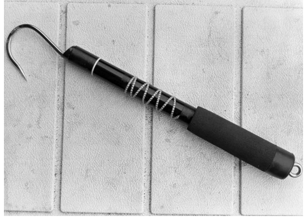
Gaff made by outdoor writer Charlie Most using a length of discarded rod blank, foam grip, and a gaff hook cemented into the end of the rod. The decorative wraps match his rods.
