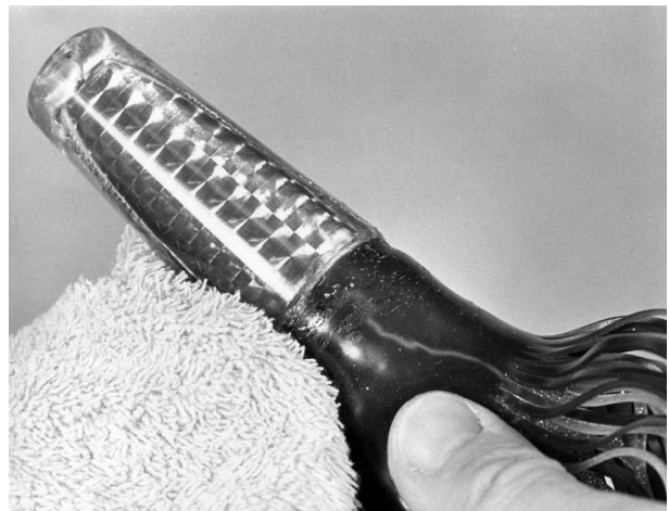
Using automobile polish to clean and polish the head after the skirt is glued in place.
