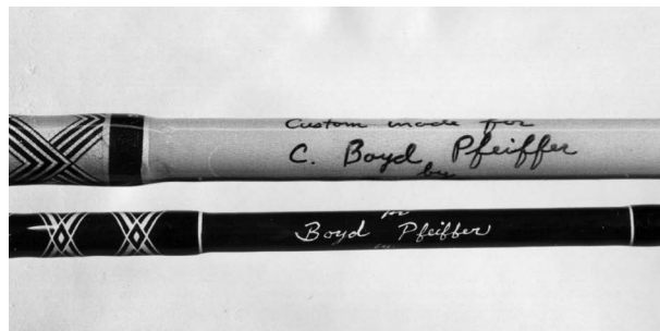
Examples of writing on a rod blank. Both white and black inks can be used, depending on the color of the blank.
