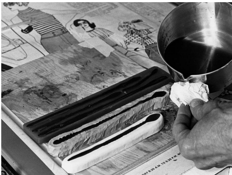
Once the molds are completely filled, use a cloth or paper towel to wipe the lip to prevent spills and drips.
