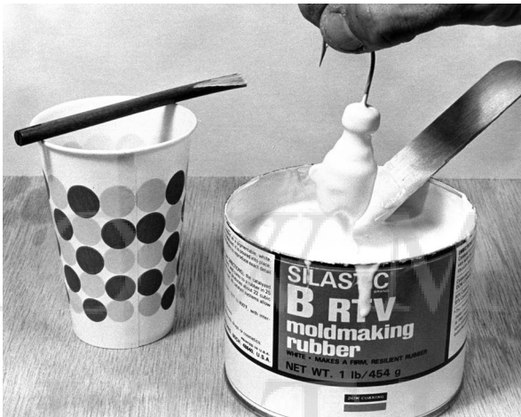
One way to prevent air bubbles when pouring the Silastic rubber is to first slowly dip the master lure into the mold compound for complete coverage. Once dipped it can be hung from a pin in a mold container, in this case a paper cup. Then the rest of the Silastic compound is added to complete the mold.
