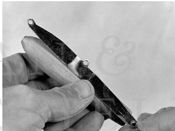
Plate being checked against the plug body for length and position of hooks.
