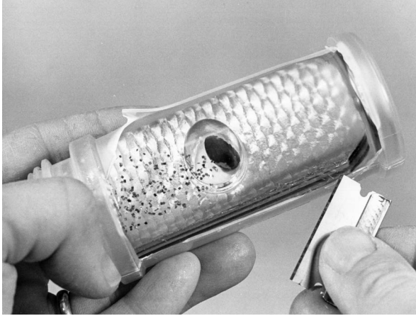
Mold partially removed, using care and a razor blade to cut away a little of the mold at a time.
