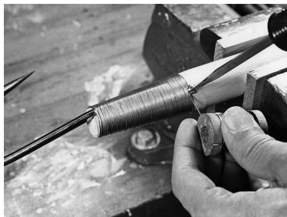
After completely wrapping the tang, the wire can be held in place using a small screw as shown.
