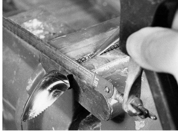
Regular stainless steel teaspoons can be used for making simple fixed-hook and swinging-hook spoons. Here a spoon is held in a vise by the handle, which has been cut off with a hacksaw.
