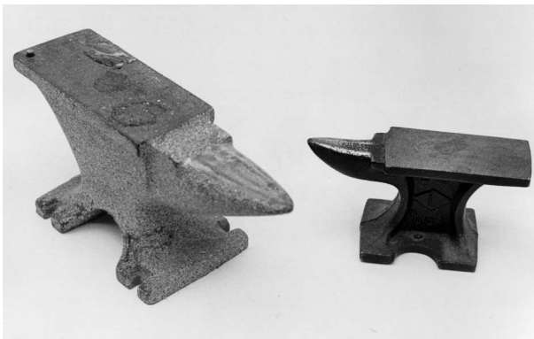
Two types of small hobby anvils for swaging lures, hammering scale marks on spoons, etc.
