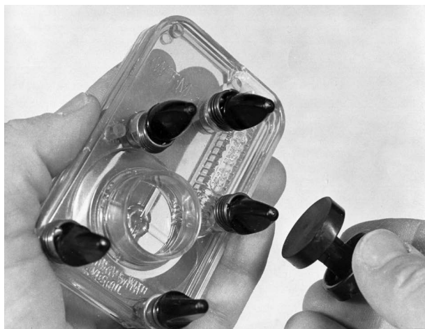
A two-piece mold from Hilts Molds for making round soft plastics. The black spring-loaded pins lock the two parts together; the plunger (right) is used to push molten plastic into the mold through an injection system.
