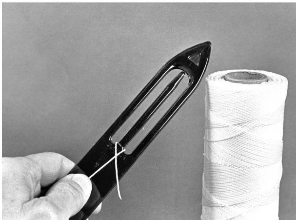
The netting cord is locked in place on the shuttle to fill the shuttle.
