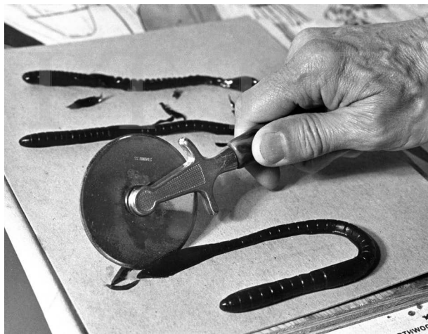
One way to salvage a lure in which the plastic has overflowed the mold is to use a pizza cutter to remove excess plastic.
