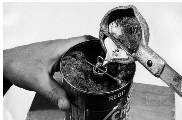
Pouring the plug retriever full of lead. Note that the plug retriever is placed in a can of sand and that the top link of chain is held in place with a nail.
