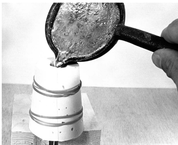
Pouring lead into the Silastic rubber mold. Note the rubber bands used to hold the two mold halves. An alternative method to using rubber bands is to mold registration pins into the mold.
