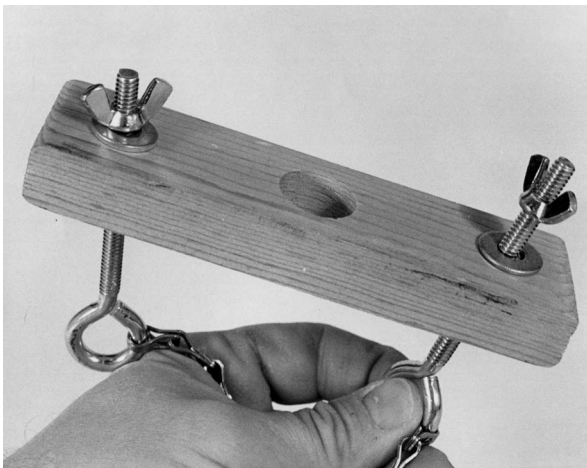
Adjustable part of the cork clamp: The rod blank can fit through the center hole, and the wing nuts adjust the pressure on the cork grip.
