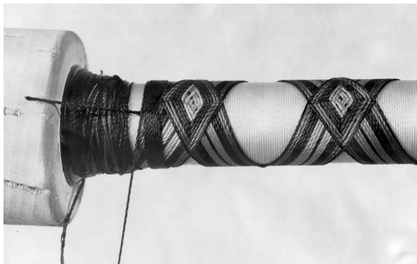
Beginning the band wrap that will hold the decorative wrap in place. This is identical to a guide wrap or underwrap, begun on the decorative wraps and worked down to the rod handle.
