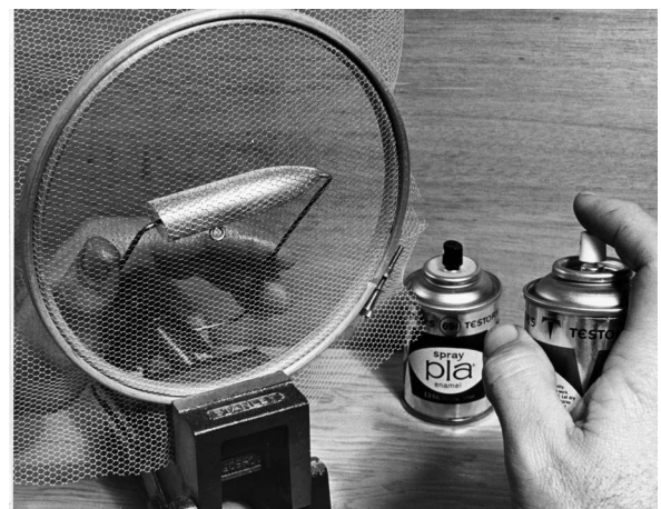
An embroidery hoop with scale netting held in a vise makes it possible to create scale finishes on lures. Hold lures tight against the netting for best results.
