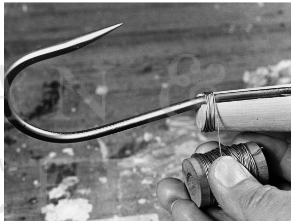
An alternative in building gaffs is to use a wood handle and wrap the end of the handle and gaff-hook tang with wire as shown.
