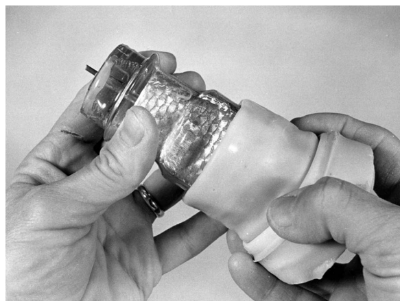
The mold being peeled off of the master lure.
