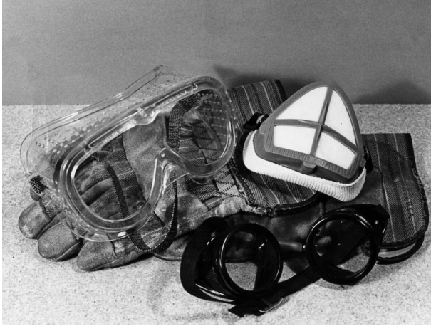
Safety equipment is very important in tackle crafting. The heavy gloves are useful for holding molds and ladles when pouring sinkers and bucktails, the facemask protects during painting, and the goggles provide eye protection for most shop and hobby operations.
