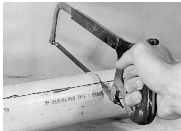
Sawing large-diameter PVC pipe for a rod case. Cut the pipe several inches longer than the longest rod or rod section you wish to carry.
