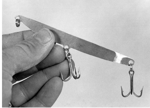
A typical plate cut from sheet metal and shaped and drilled to hold hooks and line-ties using split rings. The plate is glued into a slot in the plug.
