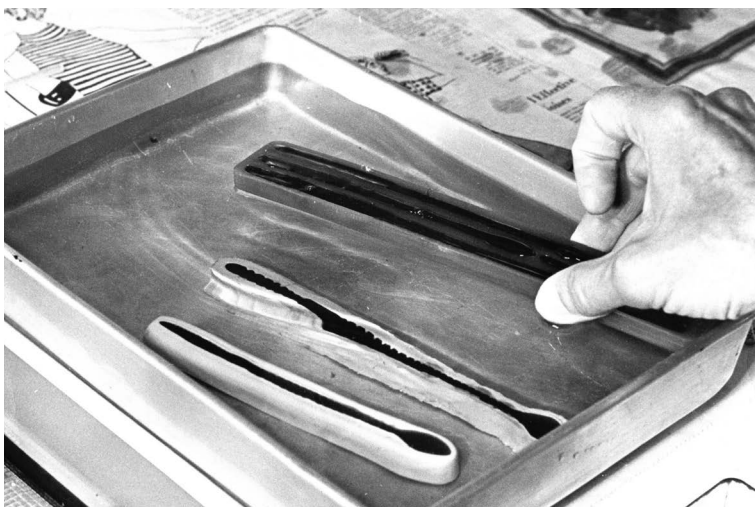
Once the molds are filled with liquid plastic, place them into a shallow pan of cold water to cure.
