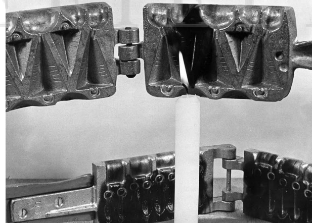
Smoking a mold with a candle flame.
