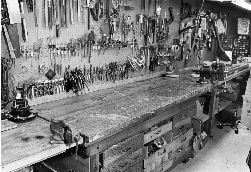
A view of the middle section of the author's workbench. Note the perfboard on the back wall to hold tools and the drawers under the workbench for tools and materials. At the far right end of the bench is a small rod-building lathe for turning handles, etc.
