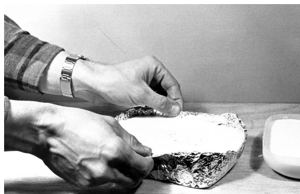
After mixing the plaster, pour it into a simple container. This mold is made from aluminum foil.
