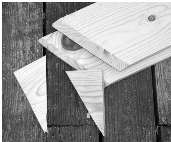
Here the boards for the side planer have been cut at an angle and sloped to make the assembled planer troll properly when used.
