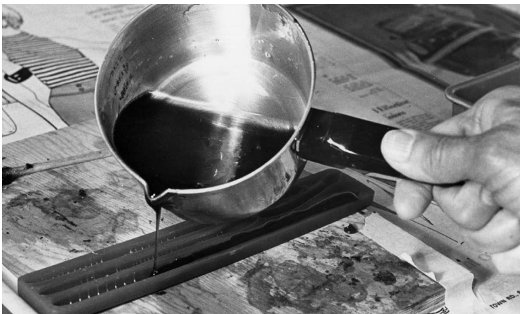
Once the liquid plastic is smooth and the color mixed in, pour into any open-face molds by beginning at one end and working to the other.
