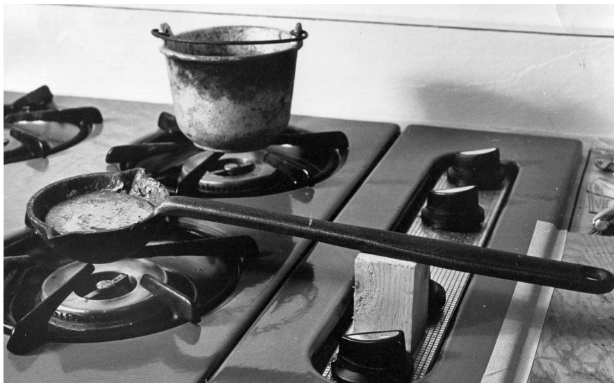
Molding requires a high heat to melt lead. If not using an electric furnace or pot, one good source is the kitchen stove, provided that proper safety techniques are used (see text). Note the wood block to hold the ladle level and the board to the right of the stove to protect the kitchen countertop.
