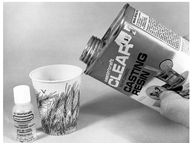
To mold, first pour out a measured amount of casting resin sufficient for the mold or molds to be filled.
