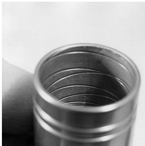
Making offshore and boat rods requires additional attention to strength in assembled parts. This gimbal butt cap from AFTCO has special grooves on the inside for additional glued strength.
