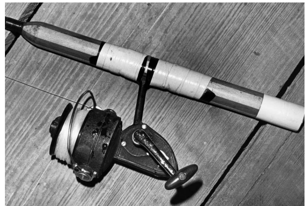
Reel seats are eliminated on some rods—the “Tennessee” handles on commercial spinning rods are an example. This similar wood handle uses a taped-on reel.
