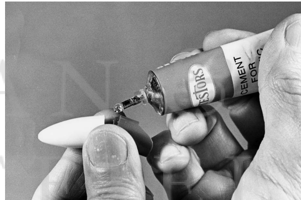
Gluing the two parts of an ultralight plug.
