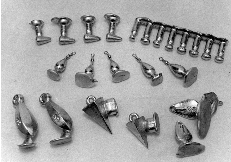
Various sinkers before the sprue (excess lead) is cut off. Wire cutters or special lead gate cutters are best for this. Since sinkers are not used as lures, no additional finishing is required.
