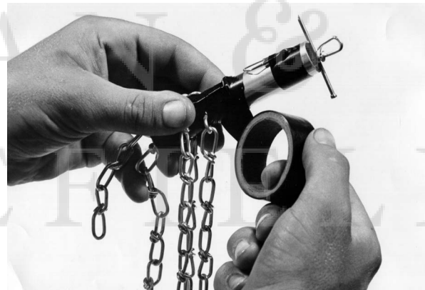
Wrapping the hole openings with tape.
