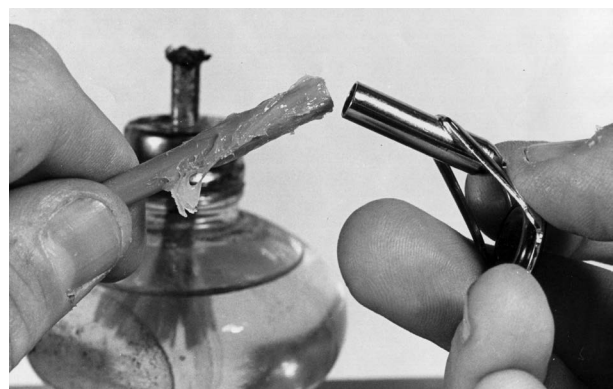
Adding tip-tops. One easy way is to melt the ferrule and tip-top cement, smear the cement on the rod tip, and immediately add the tip-top.
