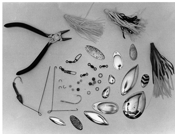
Parts for making spinnerbaits include wire forms, molded wire-form bodies, blades, hooks, skirts, split rings, swivels, beads, and clevises. In most cases only round-nose pliers will be needed for assembly.
