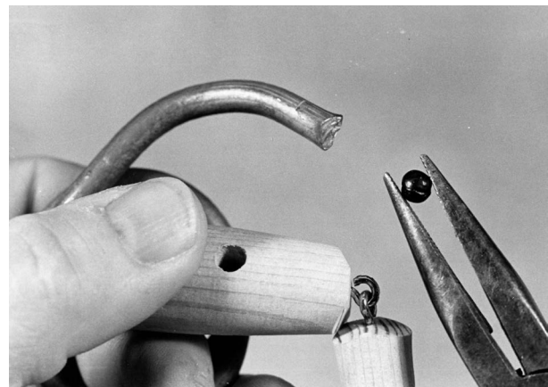
Plugs can be weighted for balance by adding pencil lead (left) or split shot to holes drilled into the belly. Molten lead can also be poured into drilled holes.
