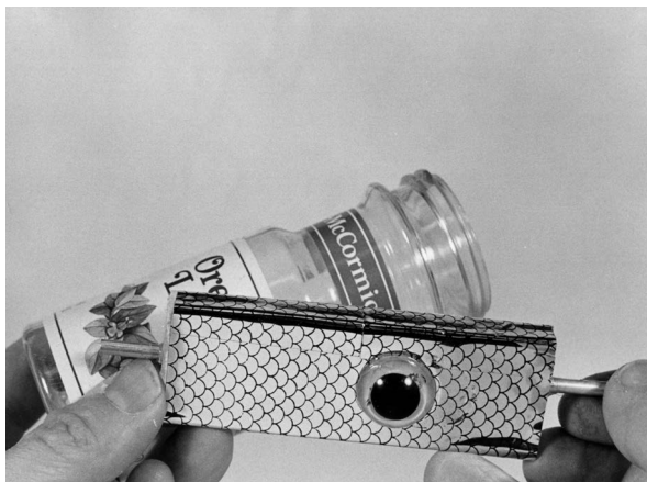
Eyes glued to a flat insert sheet, covered first with self-adhesive foil and designed to fit into a discarded spice bottle for molding the lure.
