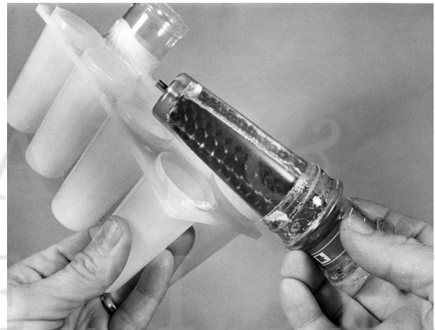
Other plastic containers can also be used for molding. Here a Popsicle tray makes tapered lures. The collar around the back, not yet removed, is from a spice bottle.
