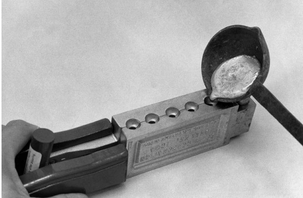
Use care to support the mold when pouring, such as is done here when using a ladle to pour an egg-sinker mold.
