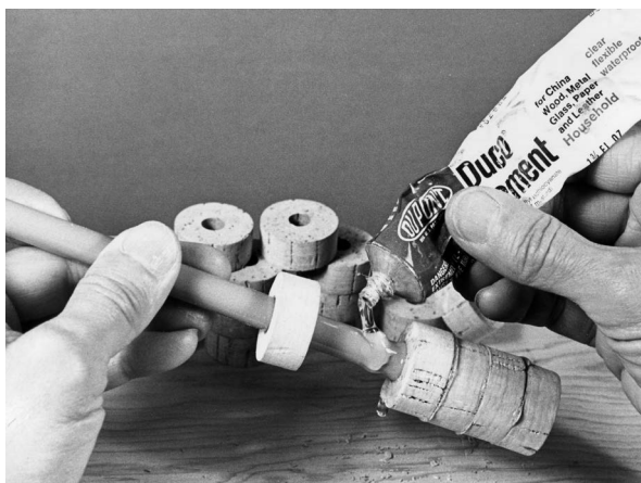
For proper gluing, each cork ring must be glued to the rod blank and to adjacent cork rings. Once all the corks are added, excess glue must be wiped off and the grip allowed to cure.
