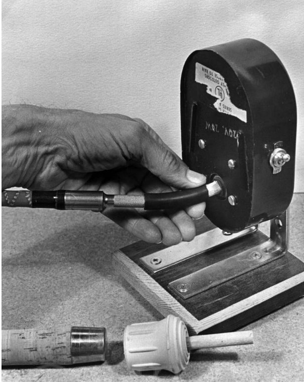
Curing motor made from a low-rpm rotisserie motor from a barbecue grill, with a wooden blind wedge in the square hole and rubber tubing to connect with the butt on a casting rod. Other types of attachment can be used, as shown by the crutch tip (to hold the rod blank or butt cap) mounted on a wooden dowel in the foreground.
