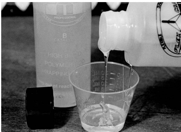
Two-part epoxy finishes require a mixing cup, as shown, for accurate measuring and mixing.
