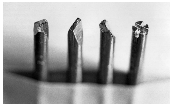
Stamping tools can be made from nails and other steel rods. These allow stamping of markings into metal blades.
