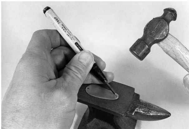
Mark the spot for drilling for the hook and line-tie attachments by using a punch on a small anvil. The punch makes a mark that will also prevent the bit from drifting or walking while drilling.
