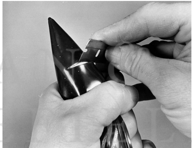
Using a razor blade to cut around the perimeter of the skirt's head for attaching to the cast plastic head.
