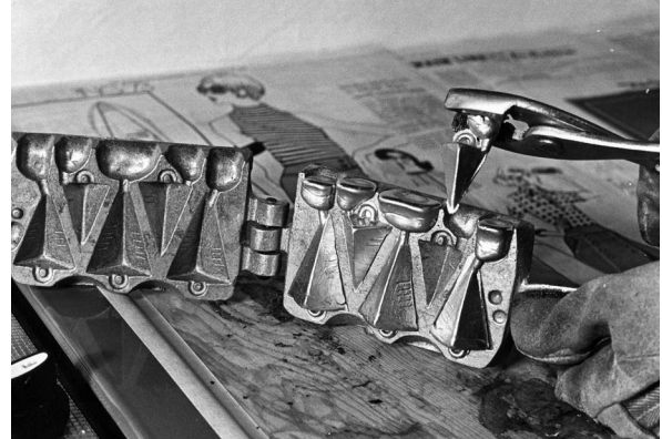
Removing sinkers from sinker mold. Use pliers, as the sinkers (and bucktails when using bucktail molds) will be very hot. Heavy gloves provide additional protection.
