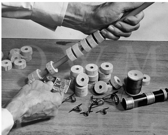
Gluing cork rings onto a rod blank.
