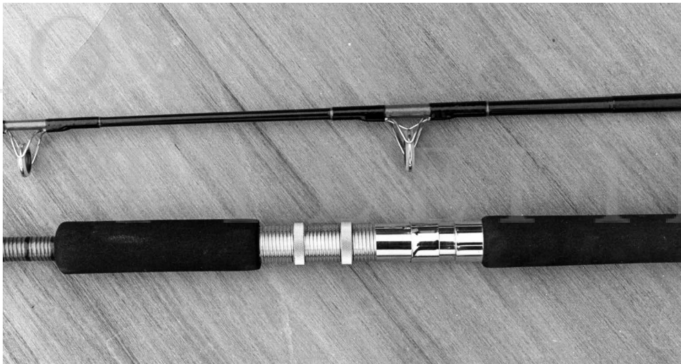
Completed basic spinning rod with simple wraps and foam handle but with a chromed reel seat in place of the graphite fill model mentioned in the text.
