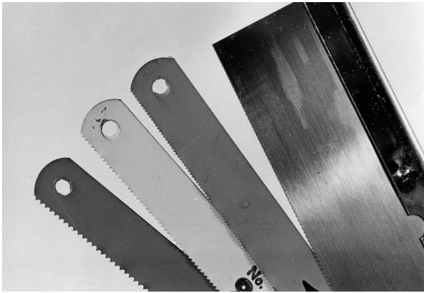
Different types of cutting blades used for tackle crafting. The three to the left are hacksaw blades; the one to the right is an X-Acto saw. Fine-tooth blades such as those with 50 teeth per inch (far right) or 32 teeth per inch (second from right) are required for cutting rod blanks.
