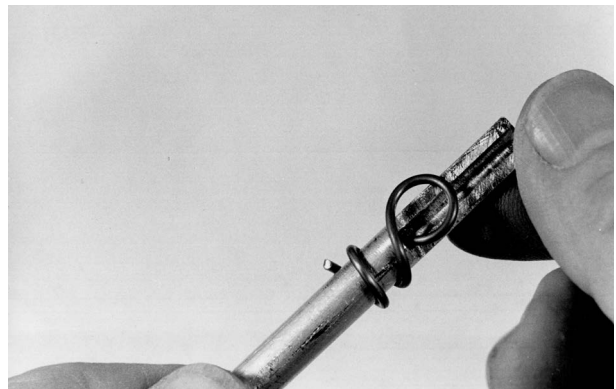
Completed pigtail wire before being removed from the wire former.
