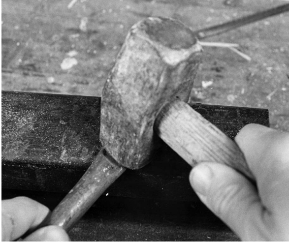
An anvil and heavy hammer are necessary for swaging flat lures from pipe. Either one or both ends can be swaged, or the entire lure can be flattened.
