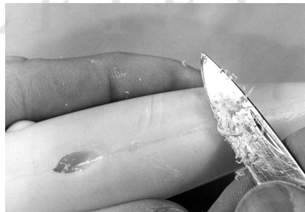
Some plastic plug bodies might need some work before painting and finishing. There may be some flash along the seam lines, easily removed by scraping with a knife.
