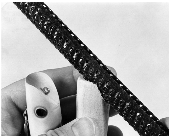
Round rasps or woodworking tools can be used to shape lips such as this sloping lip in a plug, similar to the commercial plug shown to the left.
