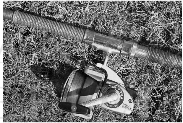
Spinning-rod handles don't have to be made of foam or cork. This handle is of wrapped heavy cord with a glued-on reel seat.
