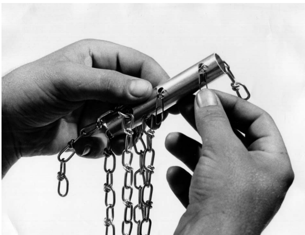
Slipping the chains into place in the drilled holes.
