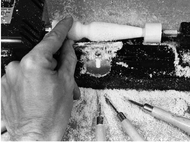
Checking a wood surface plug shaped on a lathe.
