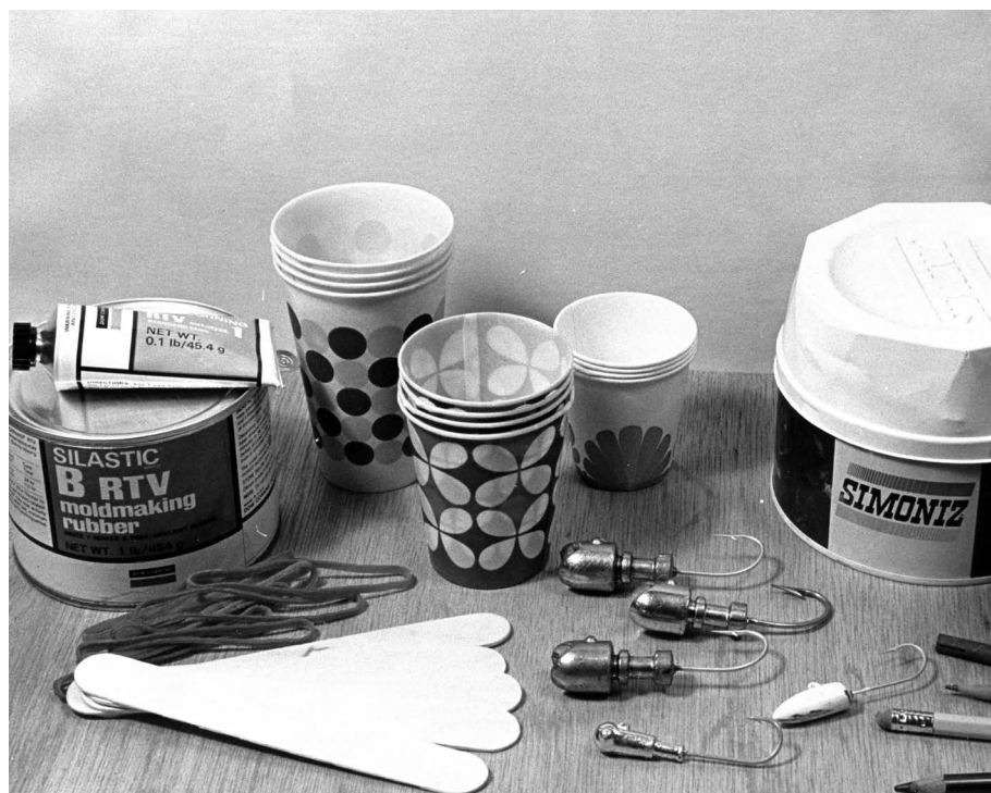
Materials and supplies needed for making molds from Silastic rubber compound. Even though these molds are made of rubber, they still allow you to mold lead lures.
