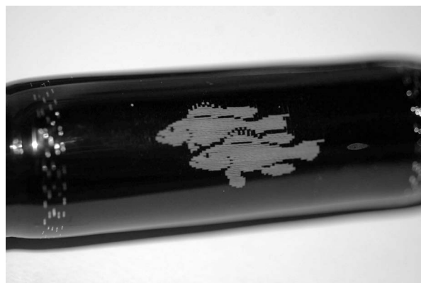
Simple weaving design of two fish woven into a butt wrap on a fishing rod.
