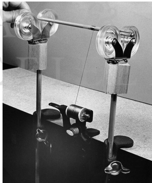
Simple thread-tension devices and rod rollers are easy to make. Here, fly-tying clamps are used to support a \frac{3}{8} -inch rod, which in turn holds short wood blocks into which are mounted plastic chair rollers. While not shown, it is best to wrap the rollers with two layers of masking tape to protect the rod and for grip for easy rolling. The thread-tension device is a standard commercial style that also clamps to the worktable.
