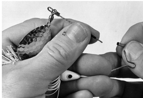
Some kits for making cable-arm spinnerbaits allow attachment of the two parts using leader sleeves, as shown. The sleeve slides onto the cable arm and is then crimped.
