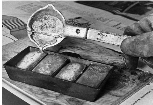
Once sinker or bucktail molding is complete, excess lead can be poured into ingot molds, available from most companies. If using a furnace or electric pot, you can leave excess lead in the pot for rapid heating next time. Check manufacturers' recommendations on this.
