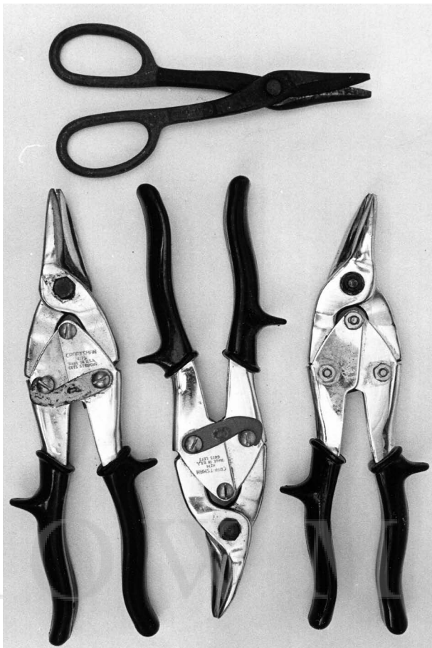
Sheet-metal snips. Top are duckbill snips. Below are three styles of aviation snips—right-cutting, left-cutting, and straight-cutting. Some snips incorporate all three cuts in one tool.
