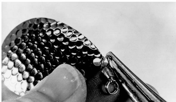
Adding a blade and swivel together with a split ring and split-ring pliers for attachment to a spinnerbait arm. Here a ball-bearing swivel is used.
