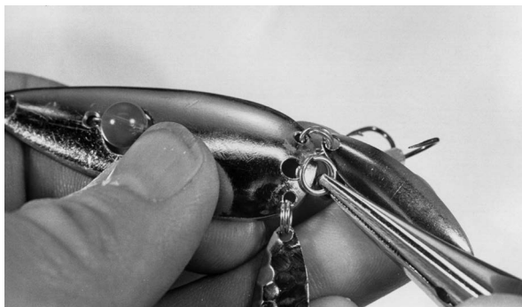
Two small spinner blades have been added to the sides of the back of this spoon for added noise and flash. The split ring for the hook is being added here.
