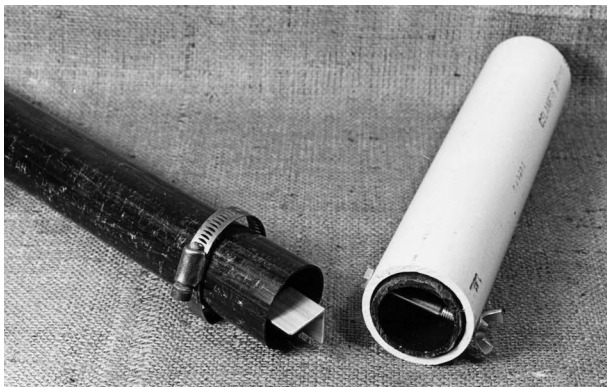
Examples of collapsible sand spikes made in two parts for easy storage in a surf bag. The parts are reversed and clamped in place to use. One uses angled aluminum held in place with a hose clamp; the other (right) consists of telescoping tubing, held in place for use or travel with a through-bolt and wing nut.
