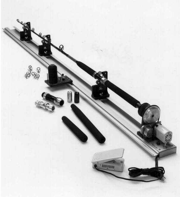
Many companies make power wrappers that are controlled by a foot pedal and turn a blank on rollers for fast, easy wrapping. This one is by Pacific Bay.
