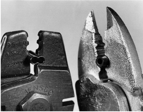
Leader sleeves (oval, left; round, right) held in place in their respective crimping pliers.
