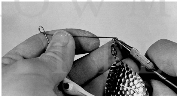
Completing the eye on the upper arm of a spinnerbait to hold the blade and swivel in place. This has been designed as a long-arm spinnerbait.
