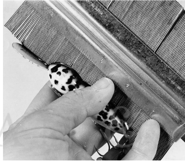
Carpenter's contour gauges can be used for copying existing plugs to make similar or identical wood plugs. Note, however, the cautions concerning trademark registration and patents in appendix B, "Sales of Tackle."
