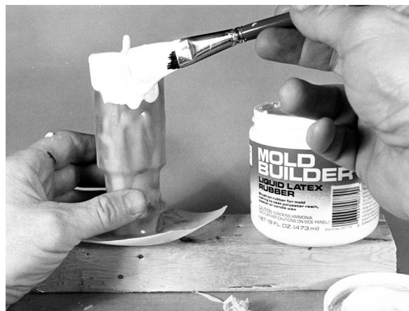
Repeated coatings of Mold Builder are necessary to give the mold strength
