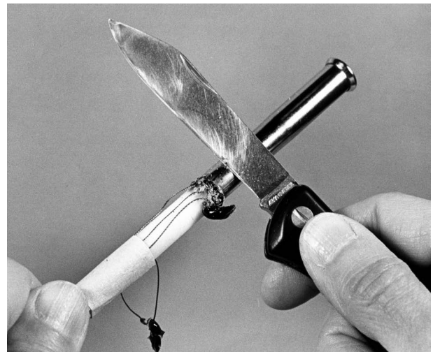
Once the ferrule cement hardens, it can be cracked off with a knife blade, as shown. This is better than trying to remove it while hot.
