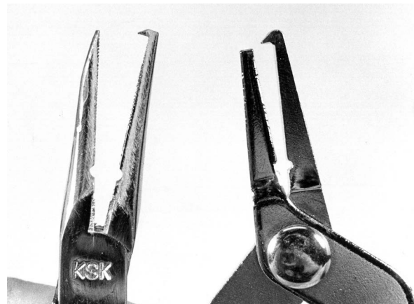
Split-ring pliers—to the left, precision pliers; to the right, an inexpensive pair. They have small teeth on one jaw to open the split ring for adding hooks and parts. The author modified the pair on the left by grinding down the nontoothed jaw to work with small split rings.
