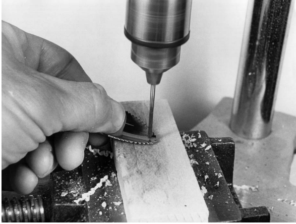
Drilling a spoon for the line-tie attachment split ring using a small hobby drill press.
