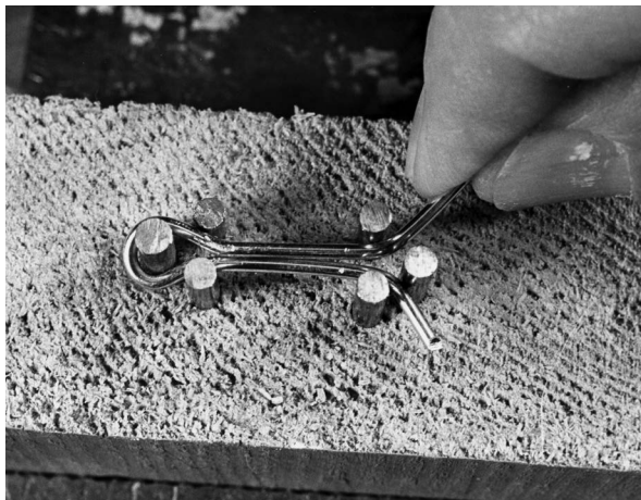
Another wire former, this one used to form the brass wire eyes used in tin squids and some saltwater sinkers.
