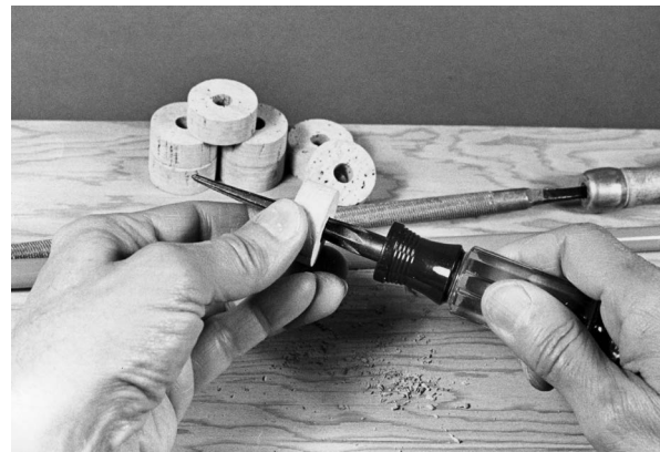
Using a reamer to ream out each cork ring to fit the rod blank.
