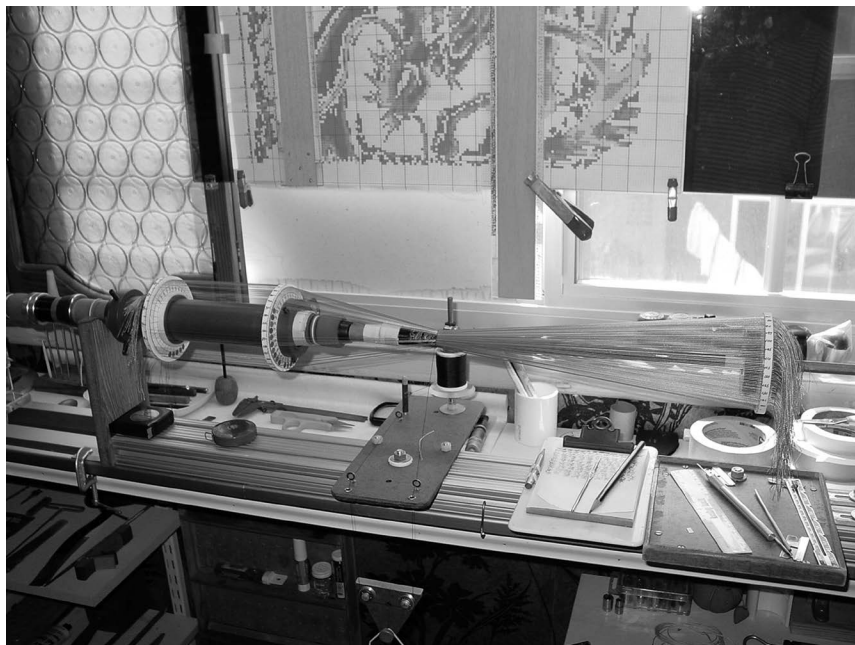
Jim Upton designed and Renzetti made the weaving machine used by Upton to weave a dragon—his specialty—onto a rod blank. Photo by Jim Upton
