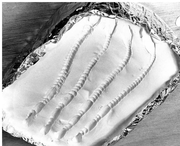
Completed plaster mold for molding worms.
