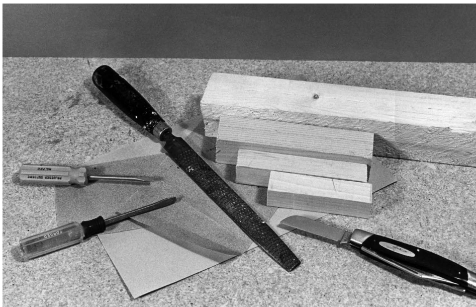
Tools and materials needed for hand-carving wood plugs. The blocks of wood are stock for making plugs. Tools include various carving and pocketknives, pliers, a rasp, and several grades of sandpaper.
