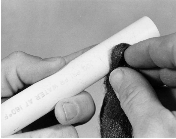
Making a plastic PVC-pipe lure first requires removing the printed markings on the side of the pipe. Steel wool is ideal for this.
