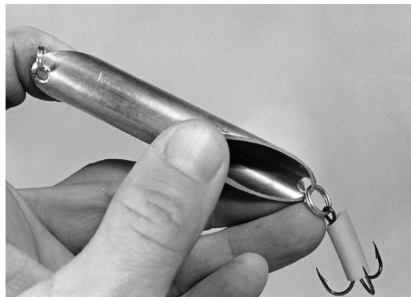
Finished metal-tubing lure, this one made from copper water pipe. The metal is strong, so no internal wire rigging is required.
