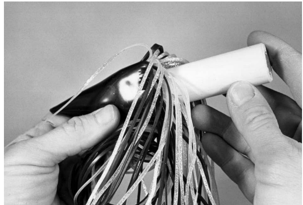
A dowel placed inside the head allows cutting the skirt at the right position for stretching and gluing onto the head.
