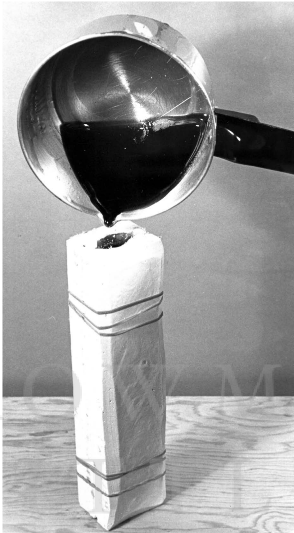
The completed two-part mold is secured with rubber bands and filled with liquid plastic.
