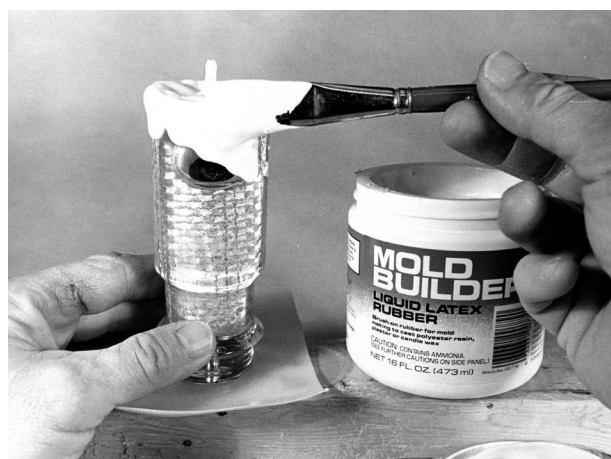
Brushing Mold Builder in place on the lure. The liquid latex is white but cures to a tan color.
