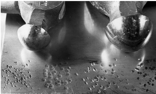
Ball-peen hammers hit on the ball, or on the side of the ball, can also make different marks in spoon surfaces.
