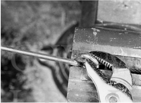
Open eyebolt to accept the chain link for the adjustable part of the cork clamp.
