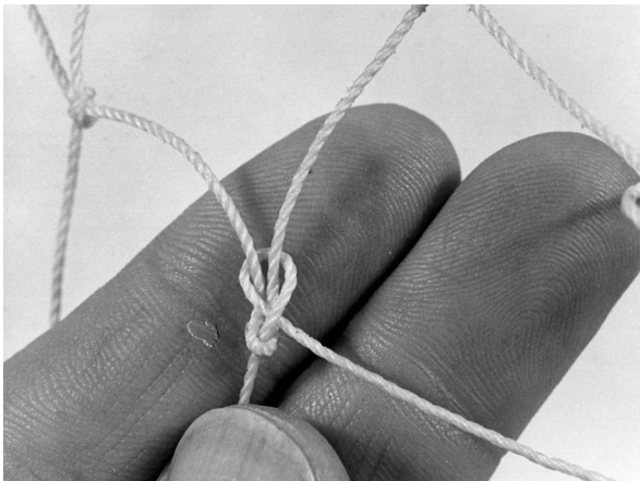
Another view of a net knot being pulled tight correctly.
