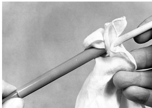
Once the sleeve is in place, glue must be removed from the ferrule. A small dowel or rod blank and rag work well for this. All glue must be removed for proper seating of the sleeve on the rod section.
