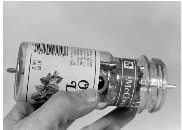
Insert sheet and tubing in the spice bottle ready for molding.
