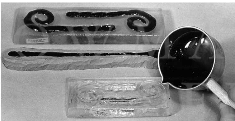
When working with curved-tail or detailed molds, begin filling at the tail or detail areas before filling the main body of the mold.
