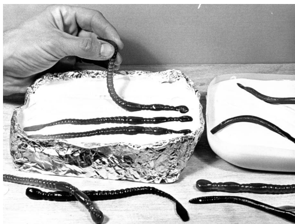
After the plaster is poured, the worms are laid in the liquid plaster. After curing, the worms are removed.
