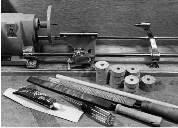
A small simple lathe can also be used for making cork grips. The tools and materials needed are shown.
