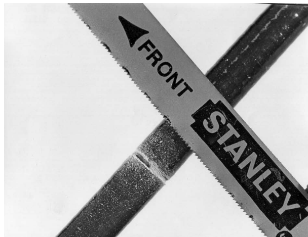
Once the blank is scored, the rod can be cut through with a fine-toothed saw.
