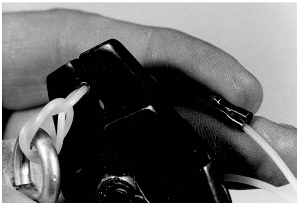
Using Mason leader pliers to crimp the leader sleeves to hold the heavy mono on the bird.
