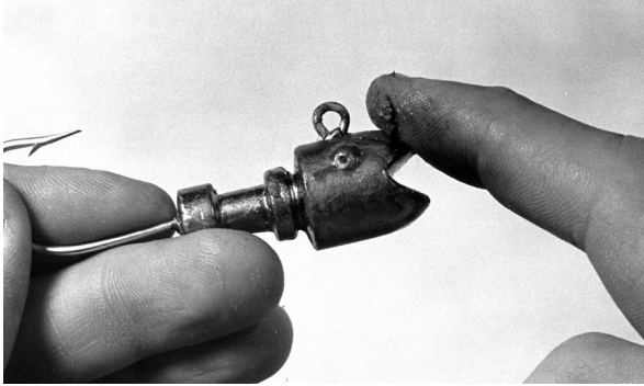
The first step in making Silastic rubber molds is to coat the master lure with a parting compound.
