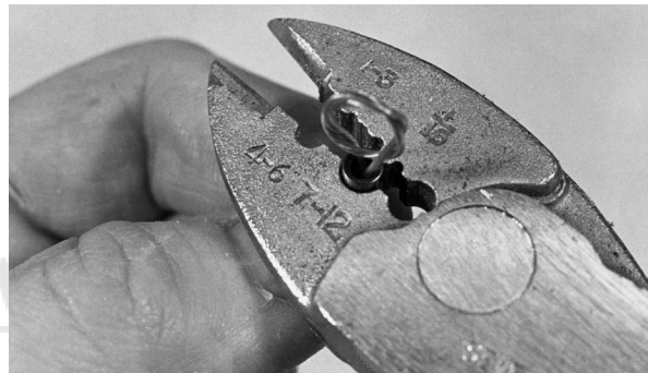
Crimped leader sleeve making a double loop in the end of a wire leader.
