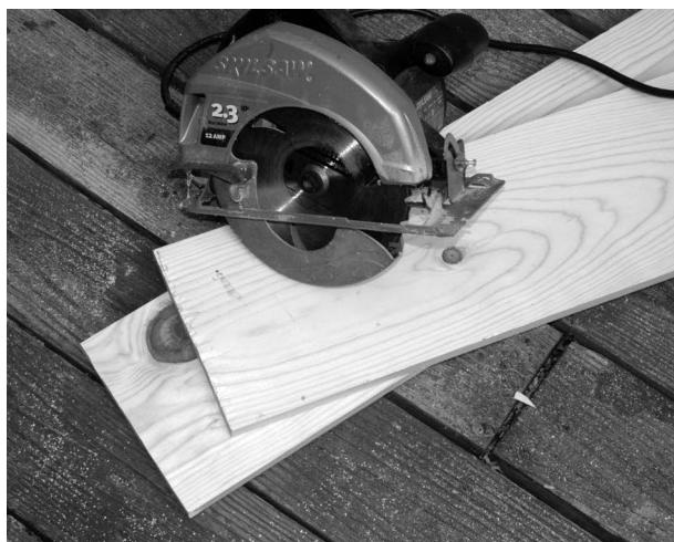
Two 1 inch x 10 inch x 3 foot-long boards with the saw used to cut and make them into a side planer for trolling more lures.
