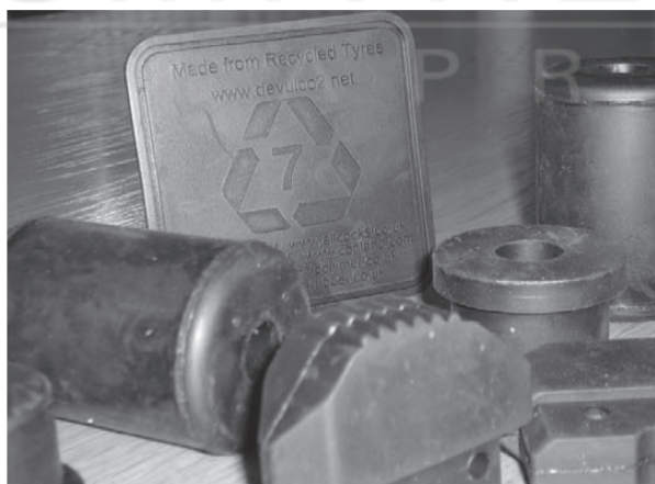
Figure 4.3 Selection of compression and transfer moulded products made from DevulCO 2 rubber. Reproduced with permission from the DevulCO 2 Project Consortium, Smithers Rapra, Shawbury, UK (Lead Partner). ©2012, DevulCO 2 Research Project Consortium
