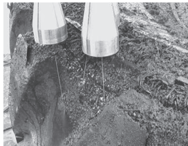
Figure 6.3 The BTRC UHP water jetting process for removing rubber from end-of-life large tyres: (a) cutting operation and (b) jetting operation. Reproduced with permission of Big Tyre Recycling Corporation, Martelaarslaan, Belgium. ©2014, Big Tyre Recycling Corporation
