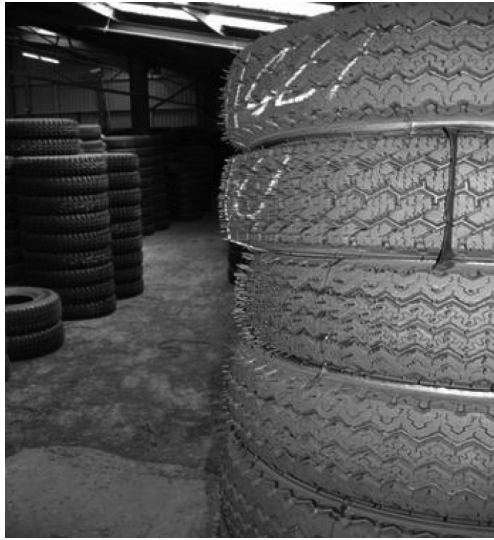
Figure 5.3 Set of cured passenger tyres retreaded with DevulCO 2 compounds waiting to be trimmed. Reproduced with permission from the DevulCO 2 Research Project Consortium (Lead Partner: Smithers Rapra, Shawbury, UK), UK. ©2012, DevulCO 2
