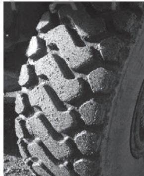
Figure 3.1 Off-the-road (OTR) tyre retreaded with compound containing 40% truck tyre 40 mesh crumb: (a) tyre carcass being retreaded with the compound; (b) moulded tyre ready for use; and (c) tyre fitted onto the OTR vehicle. Reproduced with permission from Polymer Recyclers. ©2014, Polymer Recyclers Ltd
