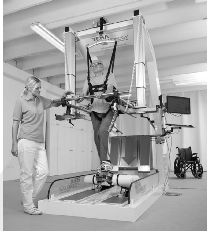
FIGURE 22.6 G-EO robot, an elliptical trainer-like gait robot that uses actuated footplates to guide and assist the user's gait.
