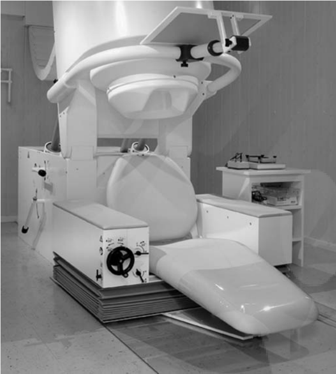
FIGURE 9.4 275-channel biomagnetometer (MEG) that measures the magnetic fields generated by neuronal activity of the brain. The magnetic fields are then analyzed to determine the neural sources in the brain and are then superimposed on an MRI image. Brain recordings can be obtained while an individual is seated or supine.
