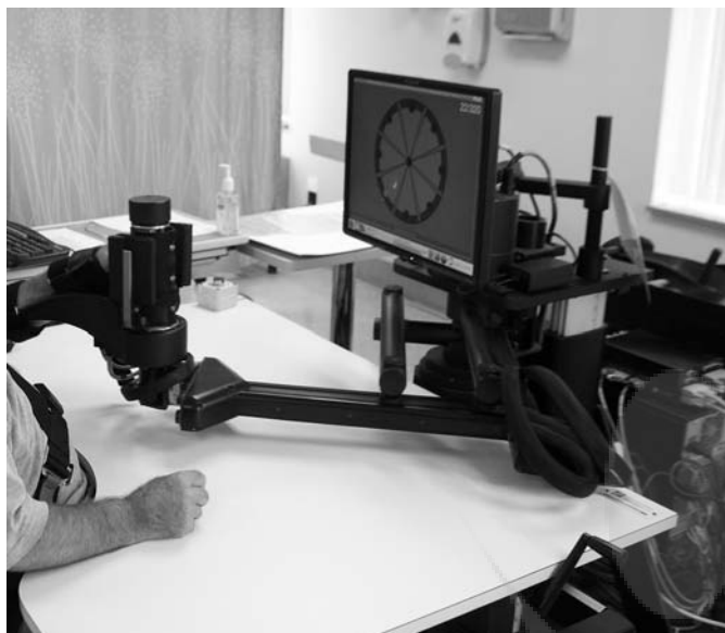
FIGURE 22.1 InMotion Shoulder-Elbow robot (Interactive Motion Technologies, Inc.), based on the MIT-Manus design, provides planar exercises for the upper limb involving shoulder and elbow movements. Shown here with the InMotion Hand robot module in use, instead of the wrist-hand splint used in the basic configuration.
