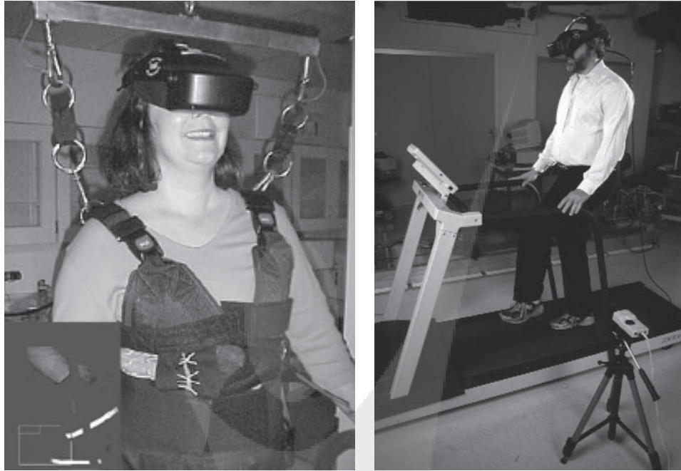
FIGURE 23.4 Participant using a head-mounted display (HMD) (left) to see a sagittal view of the leg as it is clearing an obstacle. The moving image of the leg is being captured by a single camera (right).
