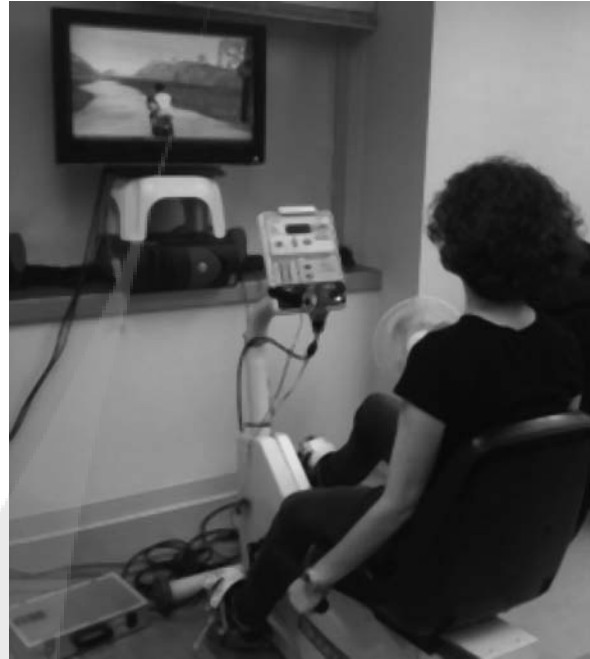
FIGURE 23.10 The Virtual Reality Augmented Cycling Kit (VRACK) converts a regular bicycle into a VR augmented cycle. It uses heart rate and pedal forces as inputs into the VE to promote both fitness and motor control.
