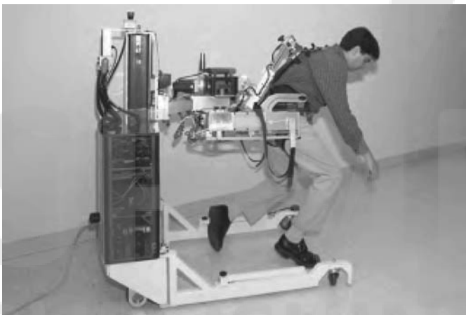
FIGURE 22.13 KineAssist (Kinea, Inc.) is a mobile robot to assist with gait training. The ability of the device to support a patient when losing balance is shown.
