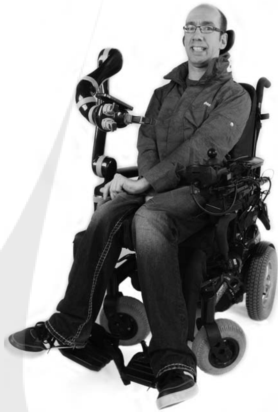
FIGURE 22.12 JACO robot arm (Kinova, Inc.) is a wheelchair-mountable ADL robot arm that assists with reaching and grasping activities.
