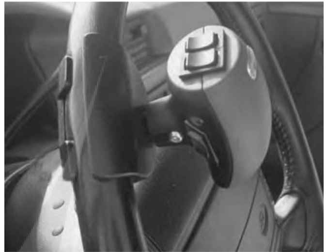
FIGURE 48.3 Spinner knob with controls (switches) for turn signals, windshield wipers, horn, and high beam.
