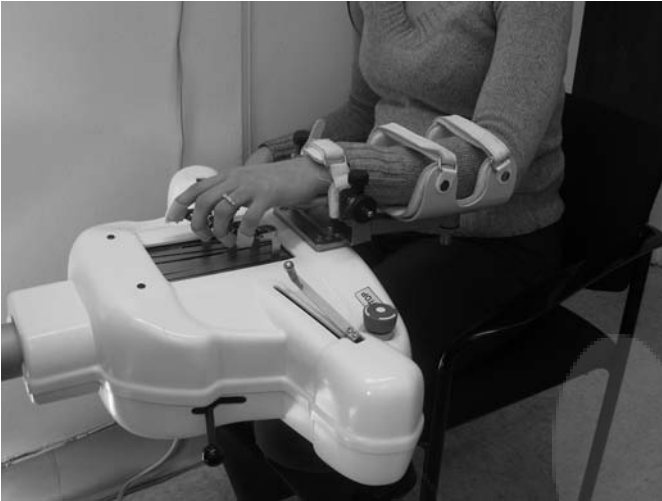
FIGURE 22.2 The Amadeo robot (Tyromotion, Inc., Graz, Austria) provides finger flexion and extension exercises.
