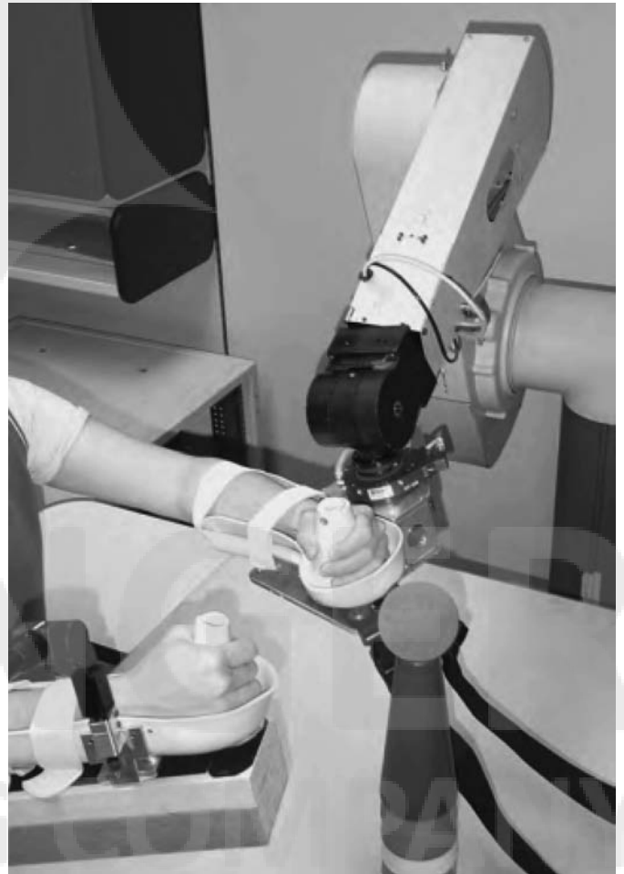
FIGURE 22.4 MIME robot, an upper-limb robot with six degrees of freedom, designed to assist with reaching movements.
