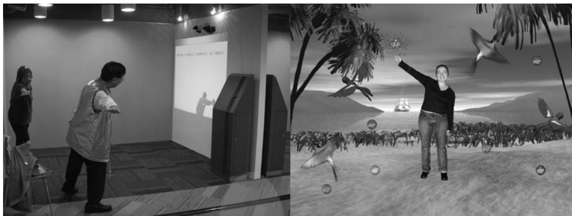
FIGURE 23.2 IREX motion capture system: on the left, participant is detected by the camera and placed into the VE. On the right, the participant's view of herself in the VE interacting with virtual objects.
