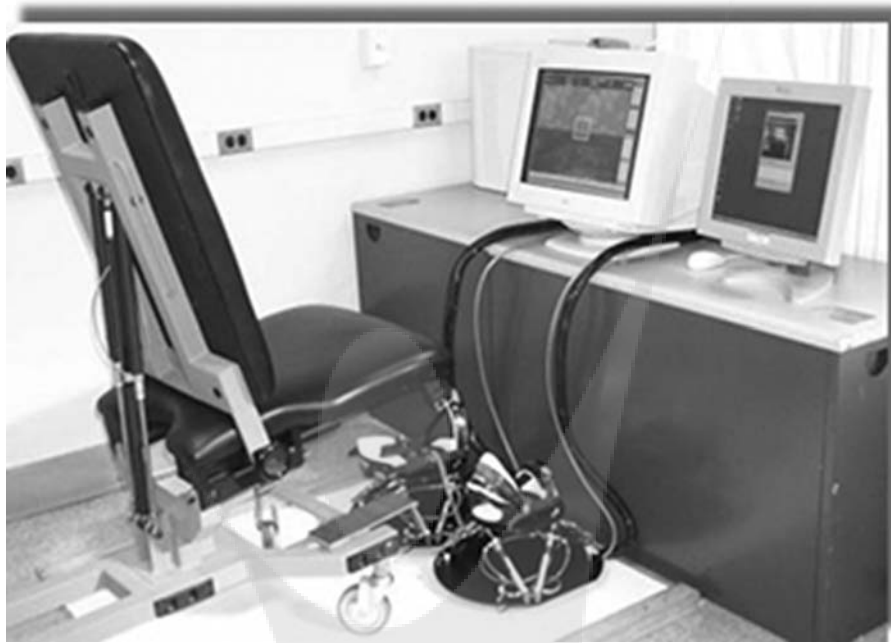
FIGURE 23.7 Rutgers ankle rehabilitation system: an instrumented robotic interface maps the movements of the lower extremity into a virtual seascape. The platform is programmed to provide haptic feedback.
