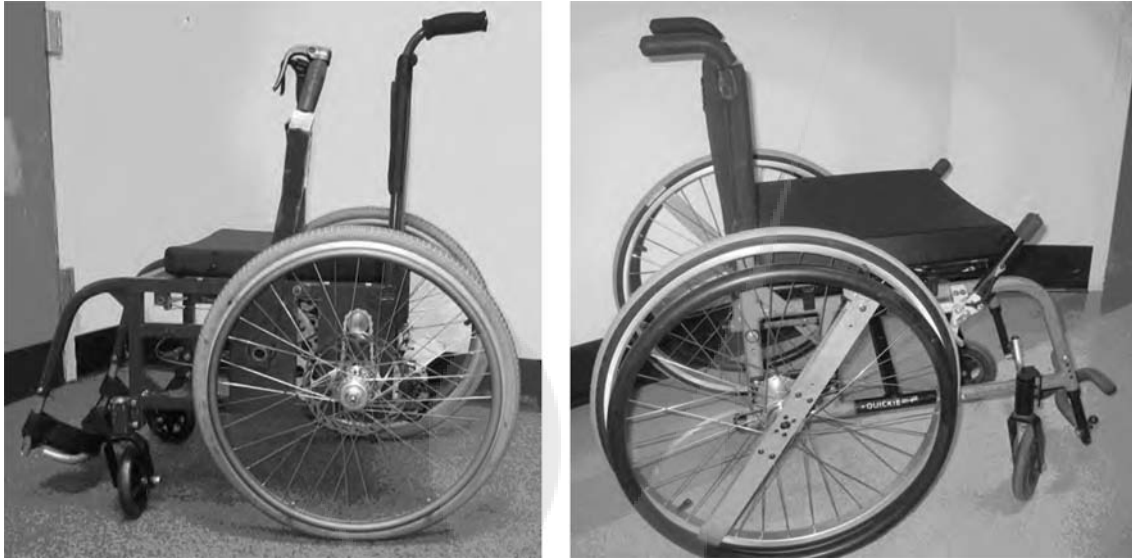
FIGURE 38.13 Lever drive system.
