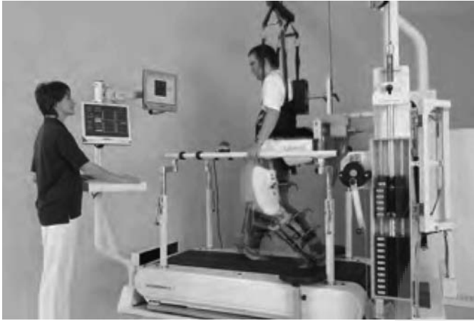
FIGURE 22.7 Lokomat robot (Hocoma, Inc.) provides partial body-weight support during assisted treadmill training.
