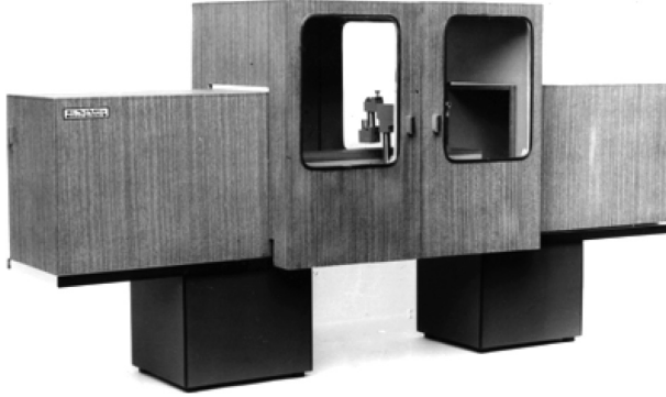
Figure 3.22. The casing of the comparator for length standards measurement.
