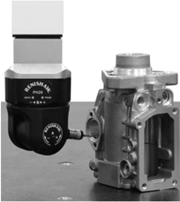
Figure 5.3. Renishaw’s PH20 touch-trigger probe CMM inspection head having facilities to rotate the stylus into the required position.
