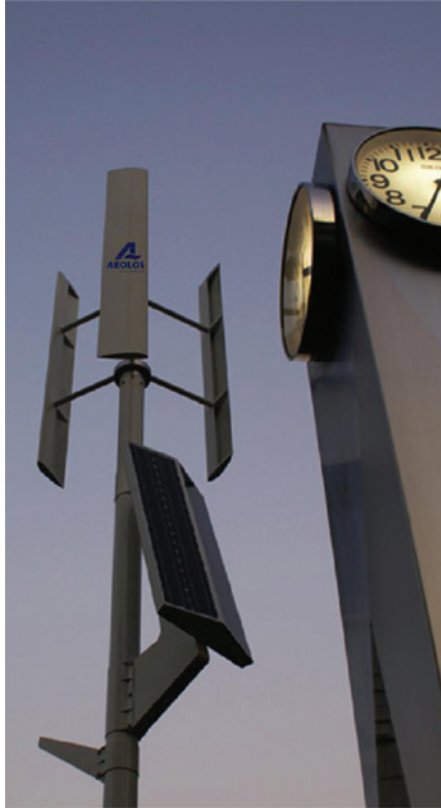
Figure 1.7. Photograph of a Darrieus VAWT connected to a solar panel, positioned in a constrained urban location.
