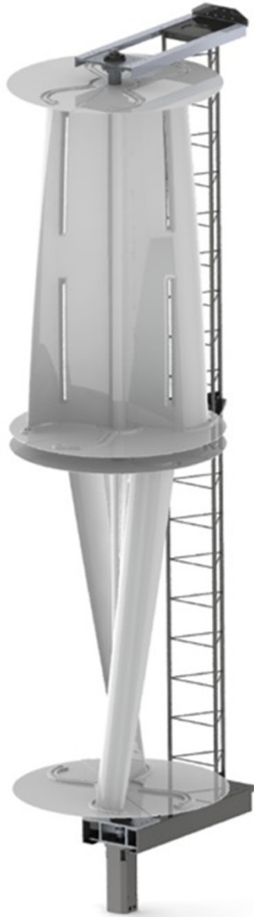
Figure 2.1. A computer rendering of a small-scale Savonius VAWT rotor.
