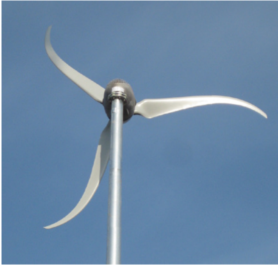
Figure 1.6. Rotating HAWT rotor with contoured blades.
