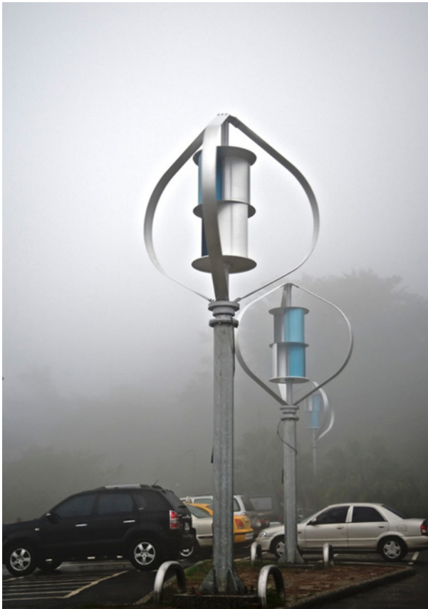
Figure 4.3. Historic Gold Mine Savonius–Darrieus combined small-scale vertical axis turbine in Taiwan (November, 2009).
