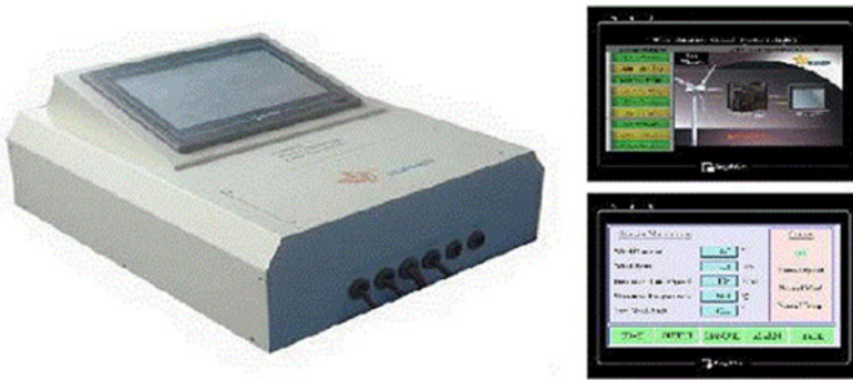
Figure 7.11. PLC Module and touch screen for easy turbine control.
