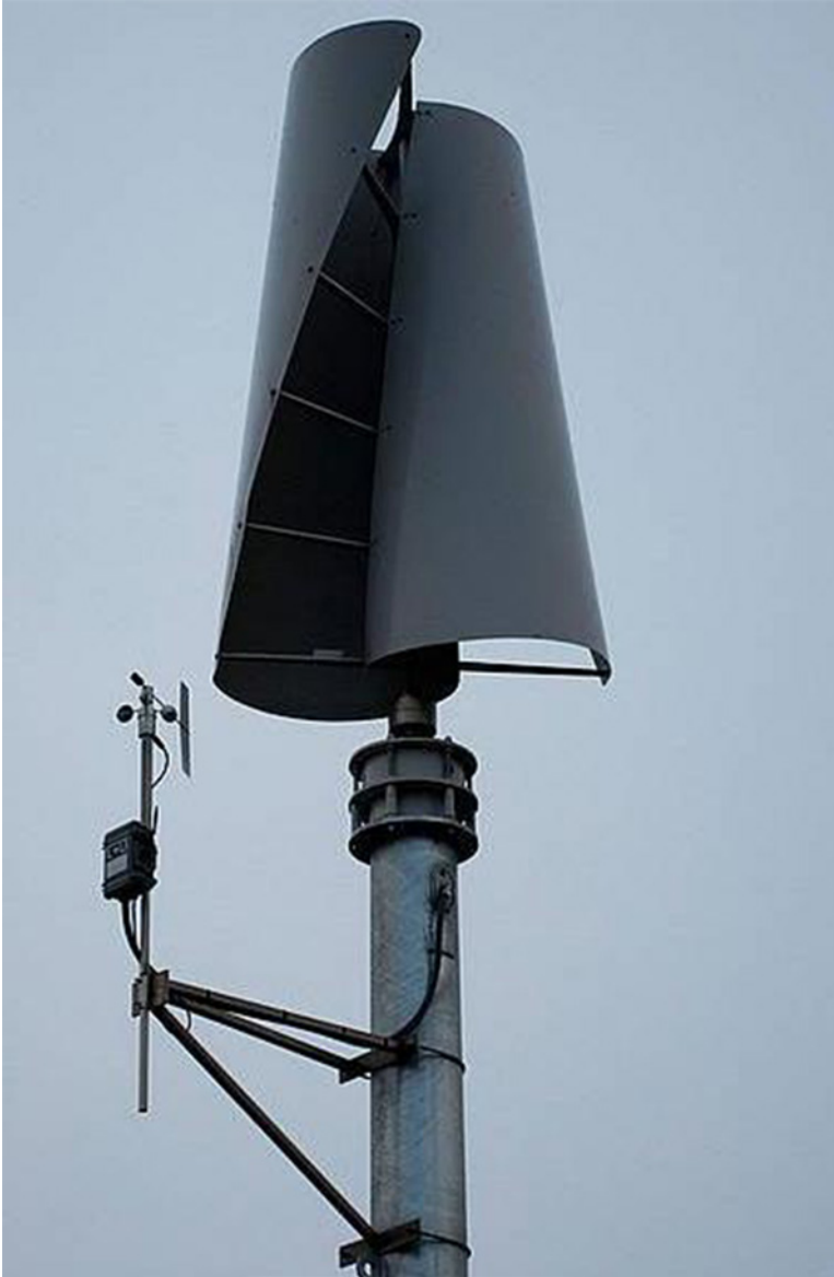
Figure 4.17. A twisted-bladed Savonius-style vertical-axis wind turbine “Gale” by Tangarie, demonstrated at Crissy Field Small VAWT Demonstration, San Francisco (2012).
