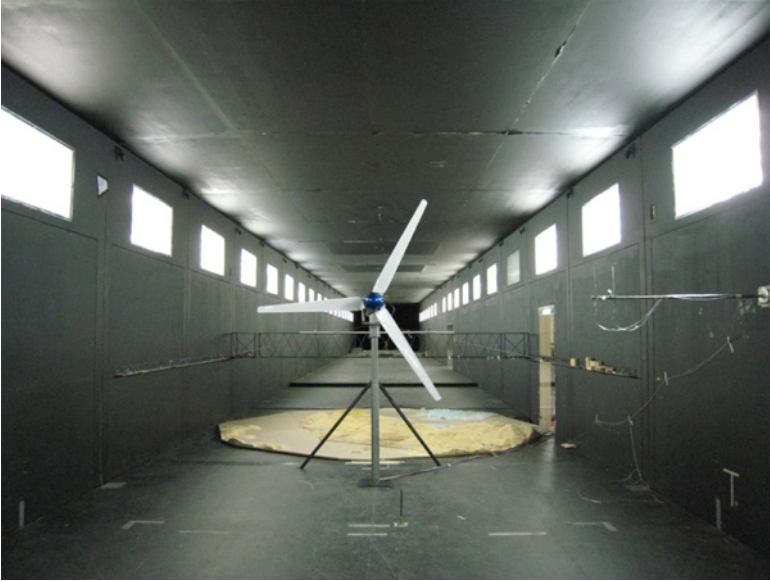
Figure 5.18. Wind tunnel test setup of a small HAWT [17].
