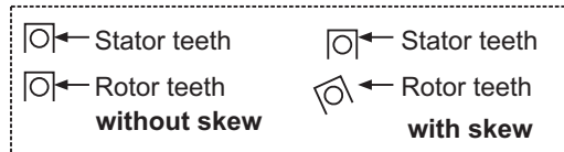
Fig. 10.3 Illustration of skewing of slot
