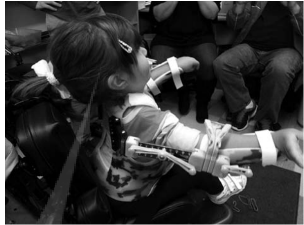
FIGURE 8.18 WREX mounted to a body jacket and constructed using 3D printed parts.
