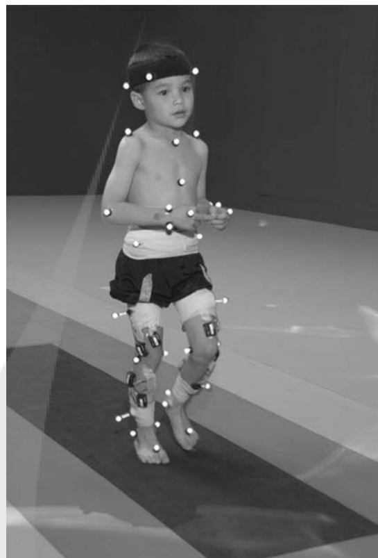
FIGURE 5.4 Subject with reflective markers or targets placed at strategic anatomic locations walks through a modern motion analysis laboratory. The location of the targets depends on the mathematical requirements of the limb-segment model used to calculate the kinematic values needed for analysis. This subject is using a full body marker set based on the Conventional Gait Model.
