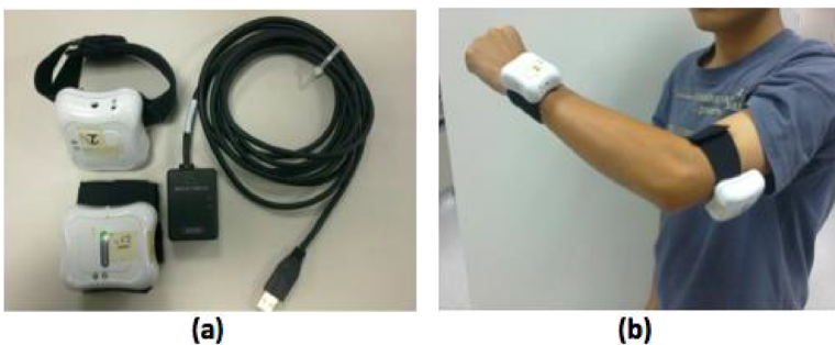
Figure 5-7 (a) The arm suit and (b) the arrangement of IMU.
