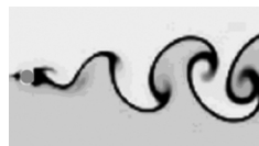
Figure 1-2 A qualitative representation of reverse Benard-von Karman vortex street produced by a flapping foil.
