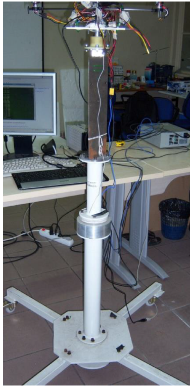
Figure 3-13 The experimental test stand that is used to experiment on quadrotor attitude and altitude control.
