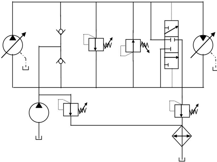
**Figure 7.29.** Rotary hydrostatic transmission circuit.
