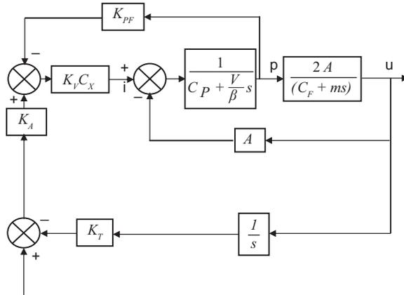
**Figure 10.22.** Pressure feedback control ( $f_E = 0$ ).
