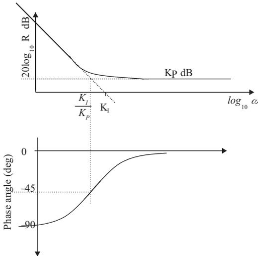
Figure 10.19. Frequency response for integral plus proportional control.
