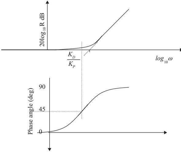
**Figure 10.20.** Frequency response for proportional plus derivative control.
