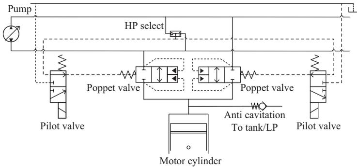
**Figure 7.35.** Pilot circuit for active control of the motor cylinder valves.
