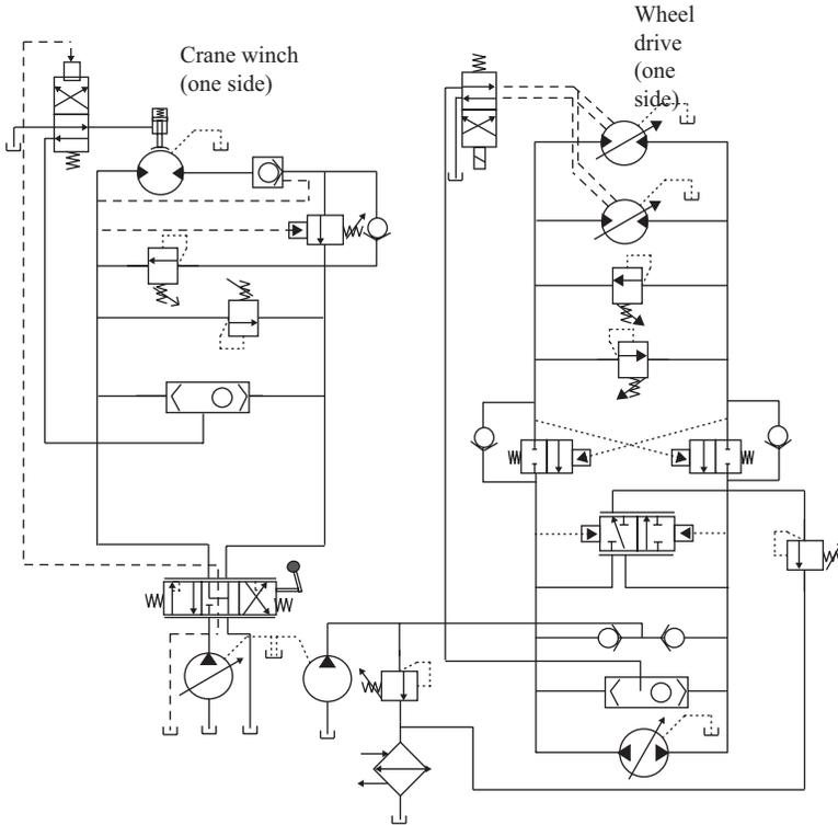
**Figure 11.5.** Circuit diagram.
