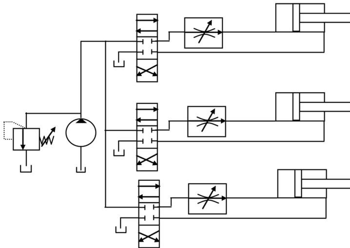
**Figure 7.14.** Multiple actuator circuit with meter-in control.
