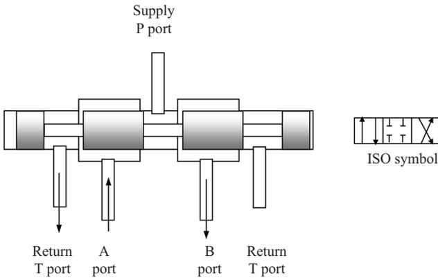
**Figure 5.1.** Four-way directional control valve (DCV).
