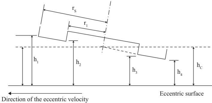
**Figure 9.5.** Cross-sectional view of the hydrostatic slipper.
