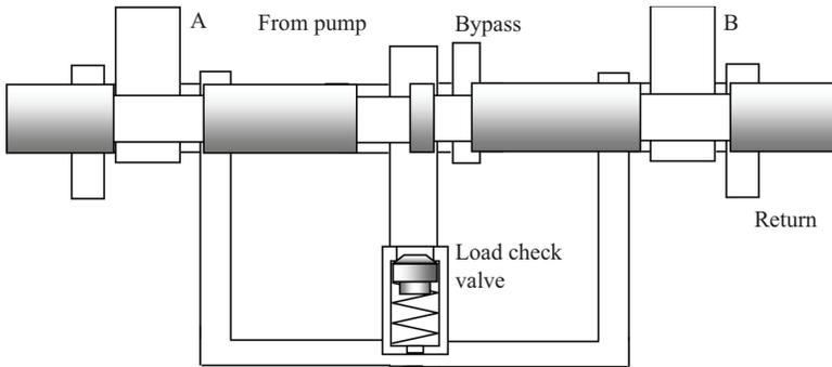
**Figure 5.8.** Bypass valve connecting the pump flow to port A and return to port B.
