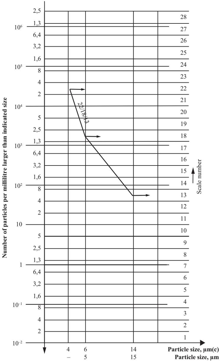
Figure 6.9. ISO 4406 standard code for contamination levels.
