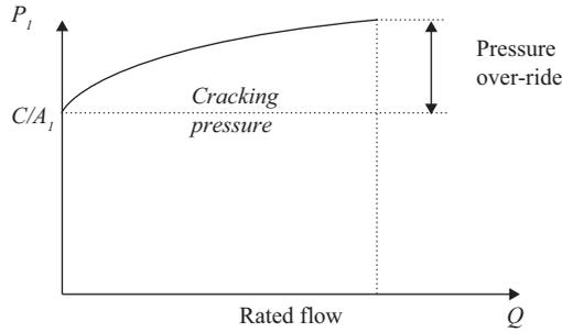
**Figure 8.7.** Valve pressure flow characteristic from Equation 8.11.
