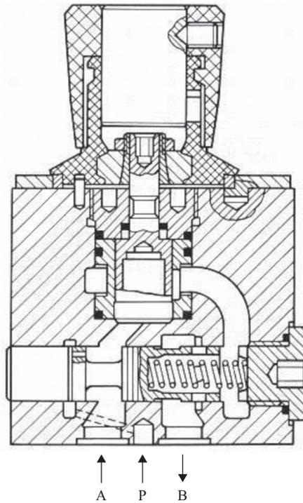
**Figure 5.6.** Pressure compensated flow control valve.
