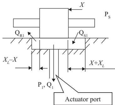
Figure 10.14. Valve underlap.
