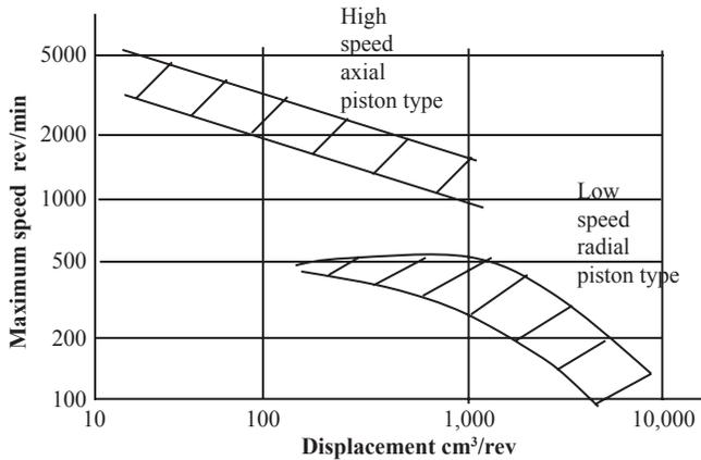
**Figure 2.14.** Typical maximum speeds for motors of various types.
