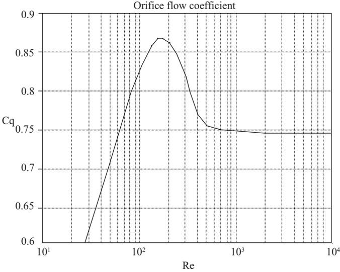
**Figure 8.5.** Flow coefficient variation with Reynolds number.
