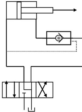
**Figure 7.9.** Actuator circuit using a POCV.
