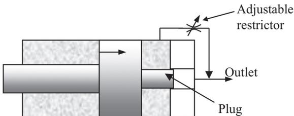
**Figure 3.7.** Actuator cushioning.
