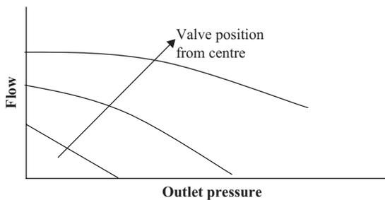
**Figure 7.22.** Bypass valve characteristics.
