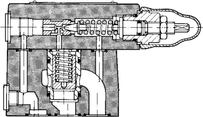
**Figure 4.2.** Two-stage poppet type relief valve.
