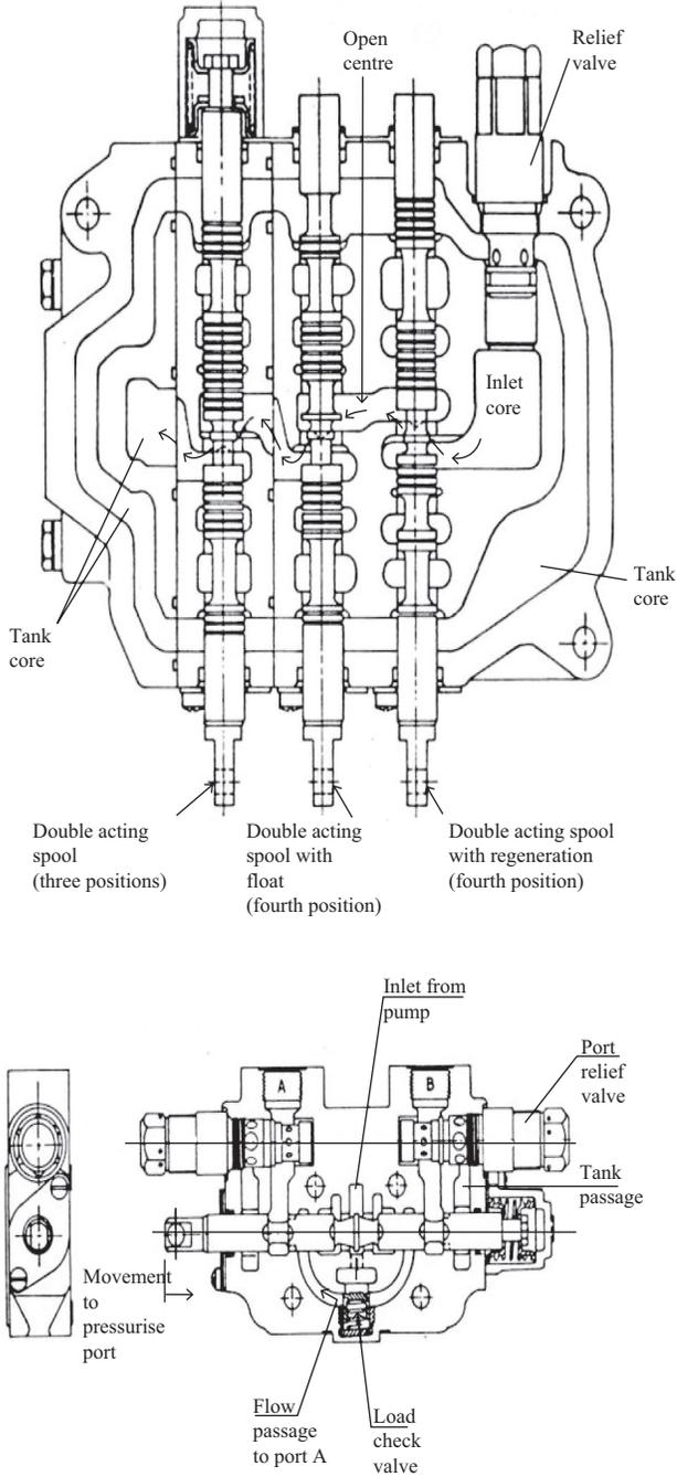
**Figure 5.7.** Central bypass valve.
