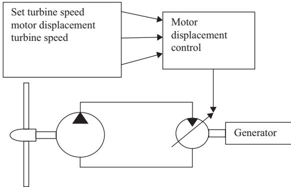
**Figure 7.36.** Wind turbine hydrostatic power transmission system.
