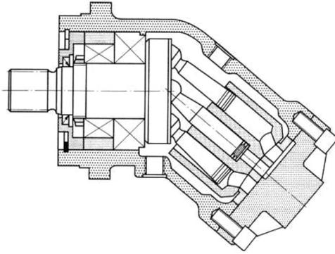
**Figure 2.7.** Bent axis type axial piston motor.
