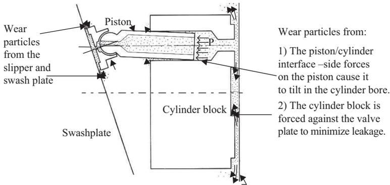
**Figure 6.5.** Wear particle generation in piston pumps.
