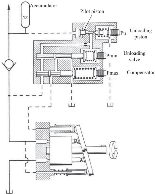
**Figure 7.28.** Accumulator charging circuit.
