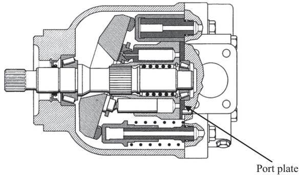
**Figure 2.5.** Axial piston variable displacement pump and motor.
