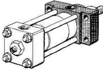
**Figure 3.2.** Actuator of tie rod construction.
