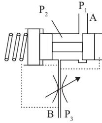
**Figure 5.5.** Pressure compensated valve.
