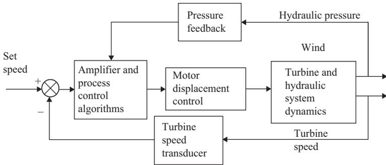
**Figure 10.28.** Turbine speed control system block diagram.
