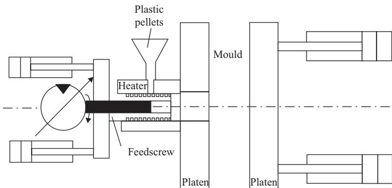
**Figure 11.12.** Injection-moulding machine schematic diagram.
