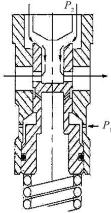
**Figure 4.7.** Cartridge type of counterbalance load control valve.
