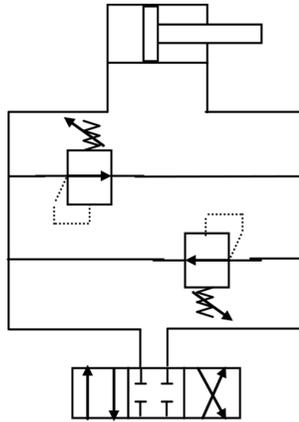
**Figure 4.4.** Dual relief valves in actuator circuit.
