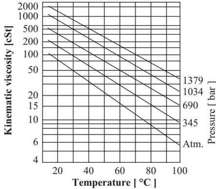
**Figure 8.1.** Oil viscosity variation with pressure and temperature.
