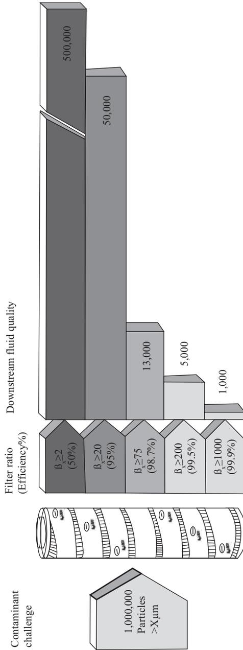
**Figure 6.8.** Downstream fluid quality and the beta ratio.
