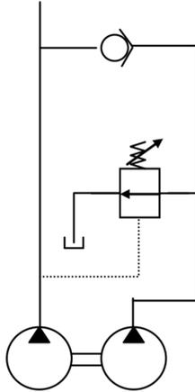
**Figure 7.38.** Double pump system with unloading valve.
