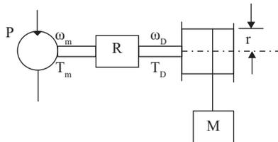
**Figure 11.2.** Winch driven by motor and reduction gearbox.
