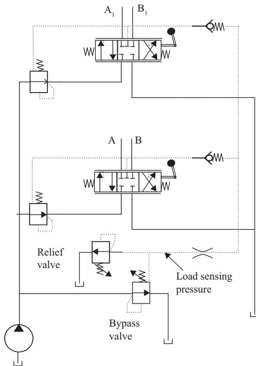
**Figure 7.24.** Pressure-compensated bypass valve with load sensing.
