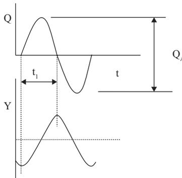
**Figure 10.10.** Sinusoidal flow variations and actuator displacement.
