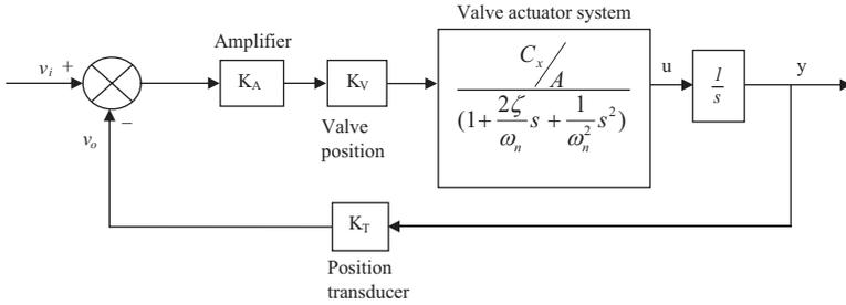
**Figure 10.12.** Electrohydraulic position control system block diagram.
