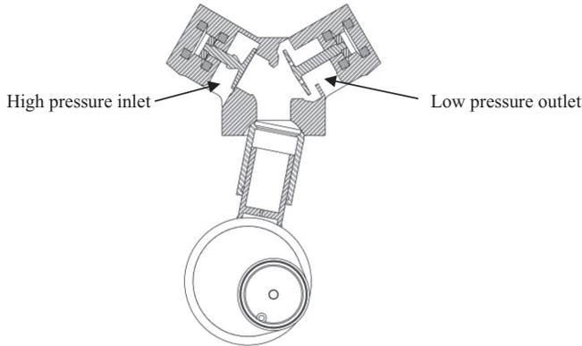
**Figure 2.13.** Digital control valves for a radial piston motor.
