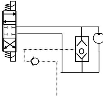
**Figure 11.25.** Alternative load sensing system.
