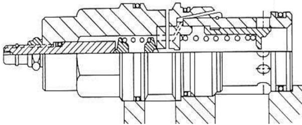
**Figure 4.3.** Two-stage cartridge relief valve.
