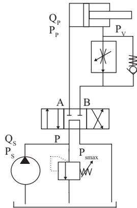
**Figure 7.12.** Meter-out control.
