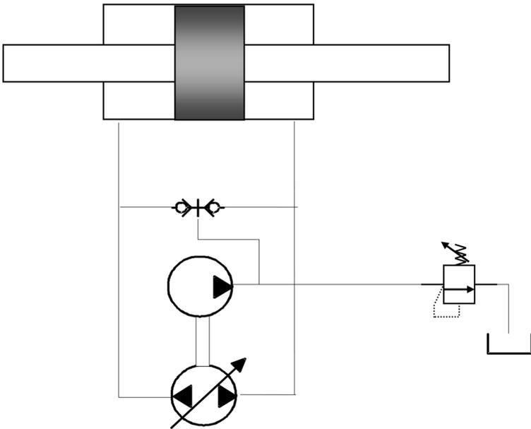
**Figure 10.29.** Actuator control using a variable displacement pump.
