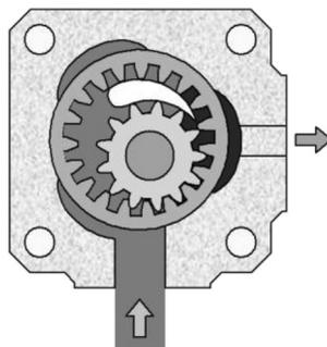
**Figure 2.2.** Internal gear pump.
