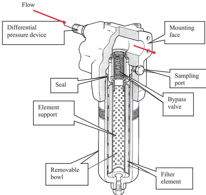
**Figure 6.6.** High-pressure filter.
