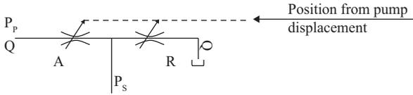
**Figure 11.21.** Hydraulic potentiometer.
