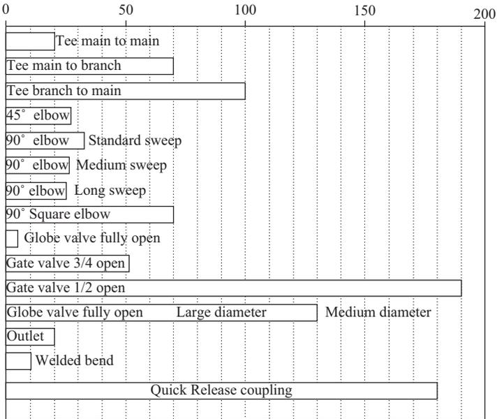
Figure 11.6. Fluid resistance in fittings.
