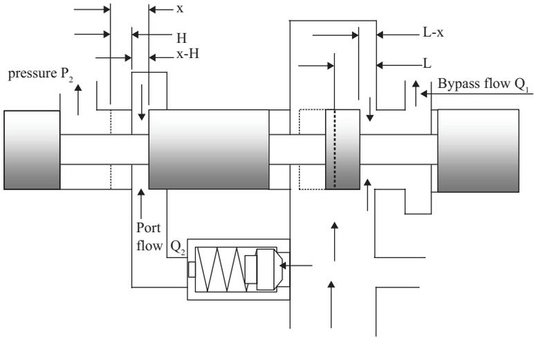
Figure 11.8. Valve dimensions.
