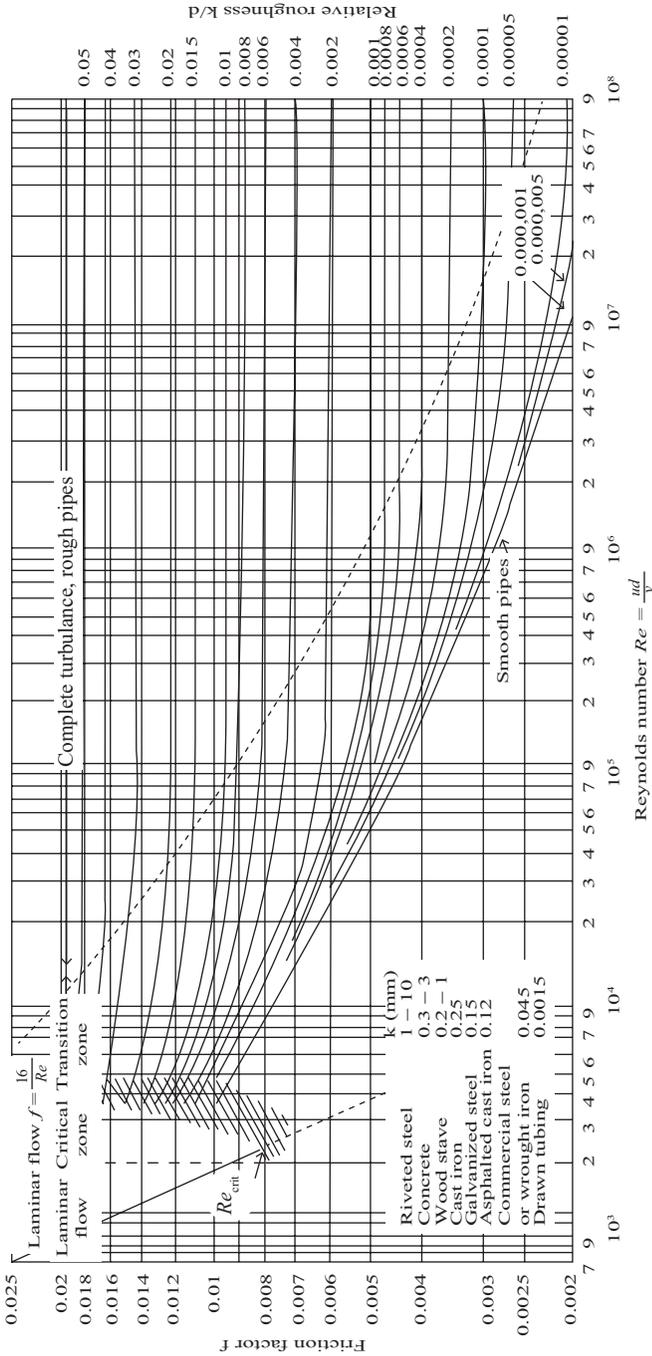
Figure 8.2. Moody chart for determining the friction factor.
