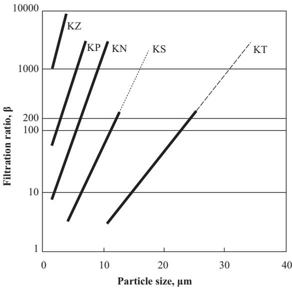
**Figure 6.7.** Beta ratio for filters.
