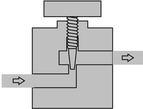
**Figure 5.4.** Adjustable restrictor valve.
