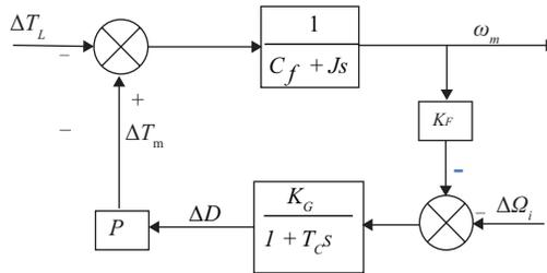
**Figure 10.25.** Block diagram for secondary control system.
