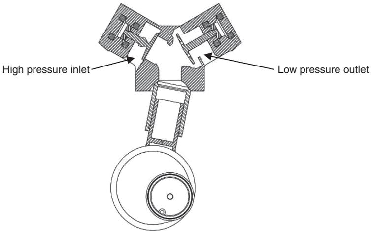
**Figure 7.33.** Radial piston motor with digitally operated valves (as in Figure 2.13).
