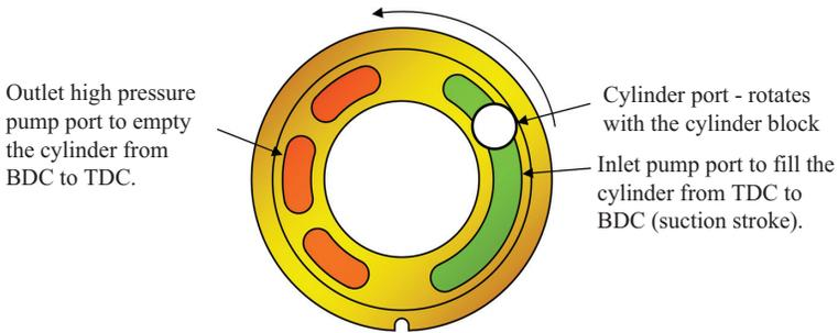
**Figure 2.6.** Diagram of a pump port plate.
