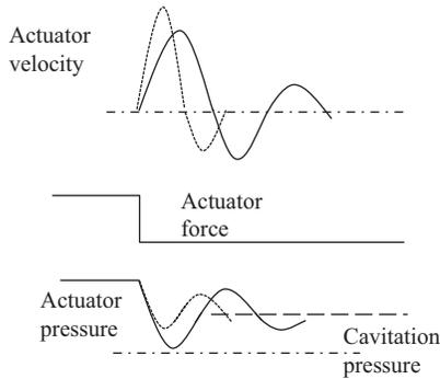
**Figure 7.11.** Pressure and velocity variations with meter-in control.
