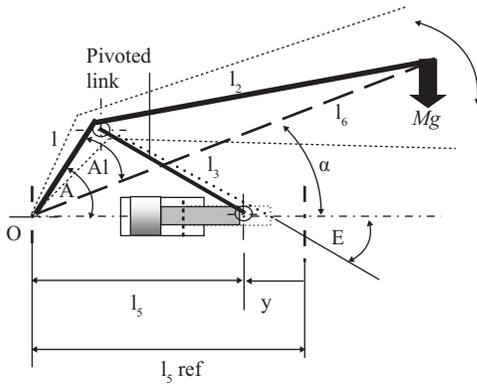
Figure 11.26. Hydraulically operated crane.
