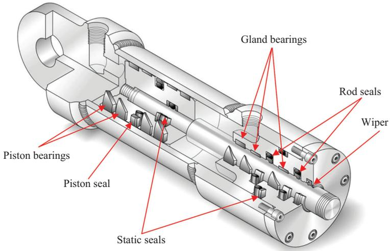
**Figure 3.5.** Section view of a typical cylinder showing the various seals.
