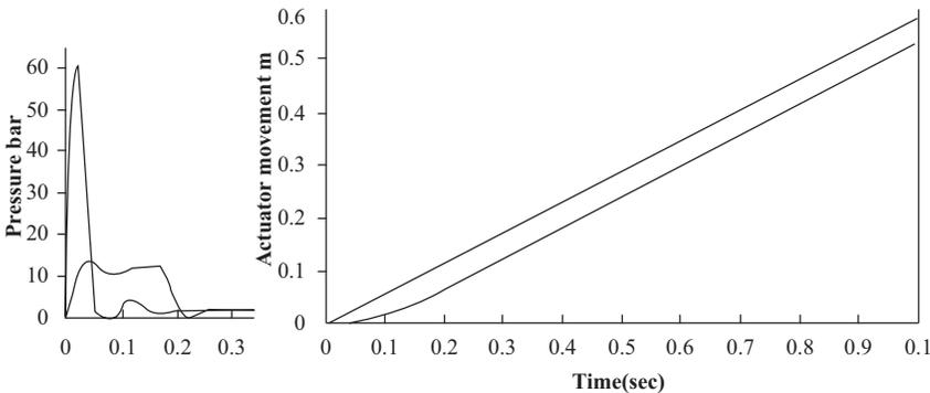
**Figure 11.14.** Variation of actuator pressure and displacement.
