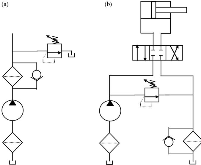
**Figure 7.41.** High and low pressure filter circuits.
