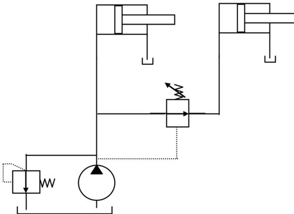
**Figure 7.39.** Sequence valve used for operation in a press circuit.
