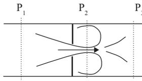
**Figure 8.4.** Sharp-edged orifice.
