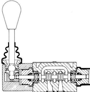
**Figure 5.2.** Manually operated DCV.
