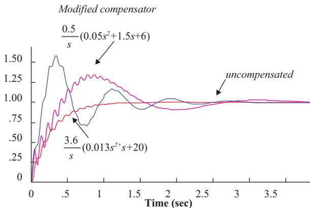
Figure 11.30. Dynamic responses using a *PID* compensator.
