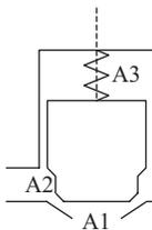
**Figure 7.34.** Poppet valve for cylinders.
