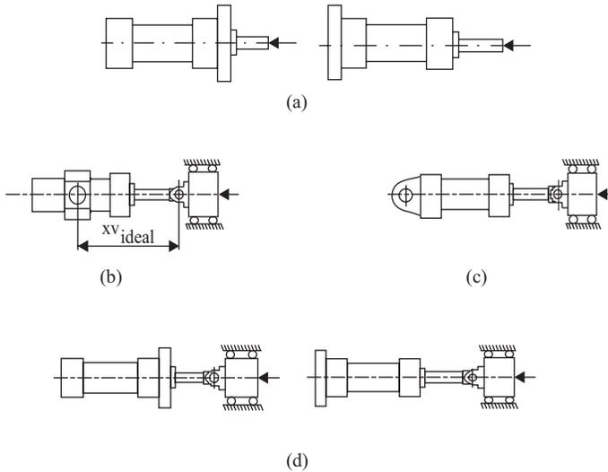
**Figure 3.4.** Actuator mounting styles (a) Actuator flange mounted to front or rear end cover with the rod end unguided (b) Actuator trunnion mounted with the rod end guided (c) Spherical coupling with the rod end guided (d) Actuator flange mounted with the rod end guided.
