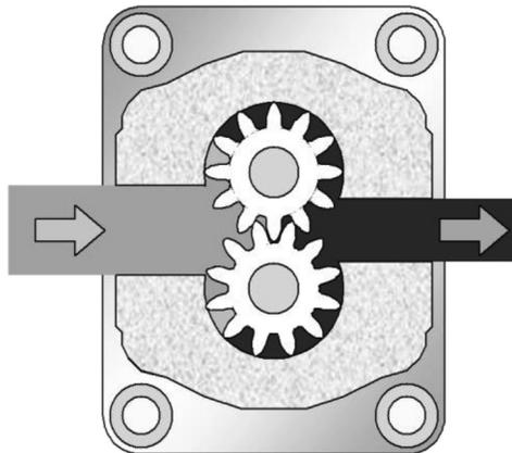
**Figure 2.1.** External gear pump and motor.
