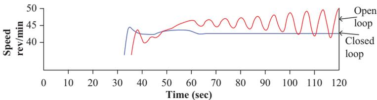
**Figure 11.33.** Nonlinear simulation of turbine speed to change of wind speed at 50 s.
