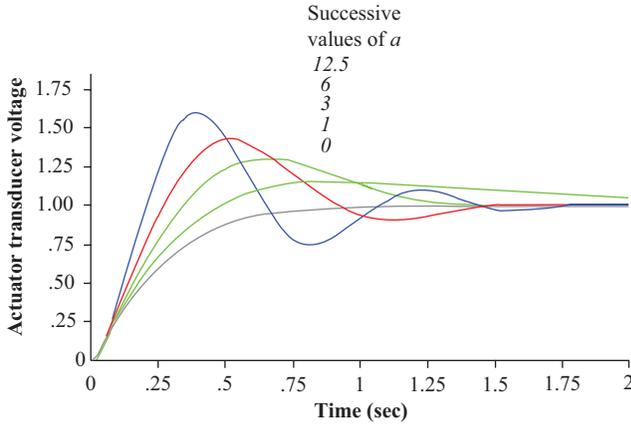
**Figure 11.29.** Step response with the P + I compensator.
