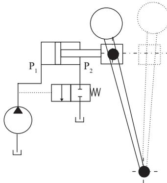
**Figure 7.37.** Load control circuit using counterbalance valves.
