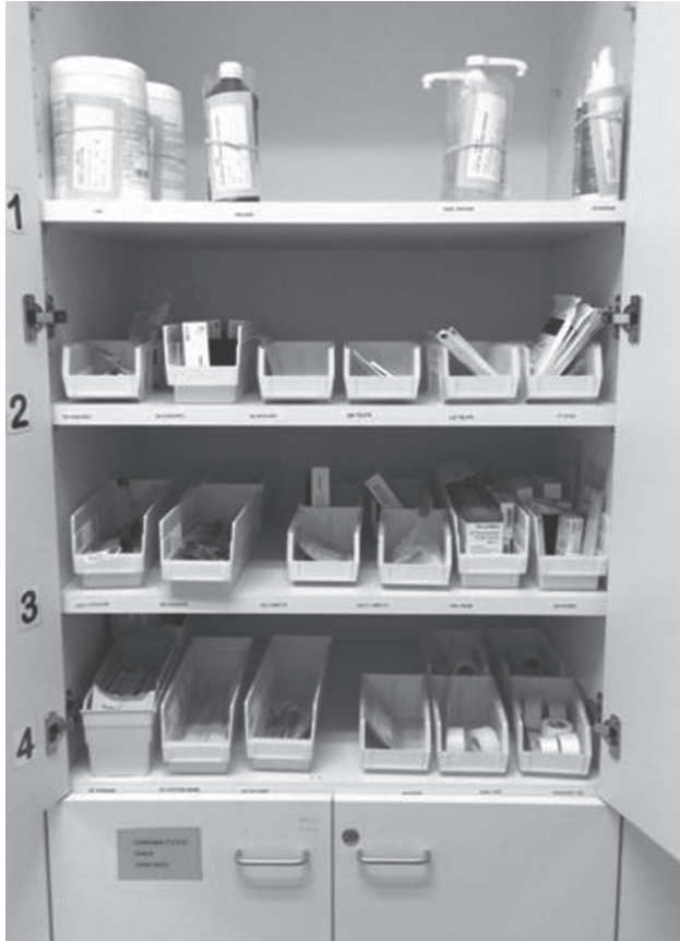
Figure 1.19 The result of the stock cabinet after the improvement project. The cabinets now have bins with labeled locations, and the shelves are labeled to create a standard location for each item, which is easily replicable by whoever restocks the cabinet or uses supplies
