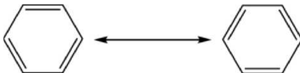
Figure 3.9. A benzene ring. This six-carbon ring is the basis of many common aromatic compounds
