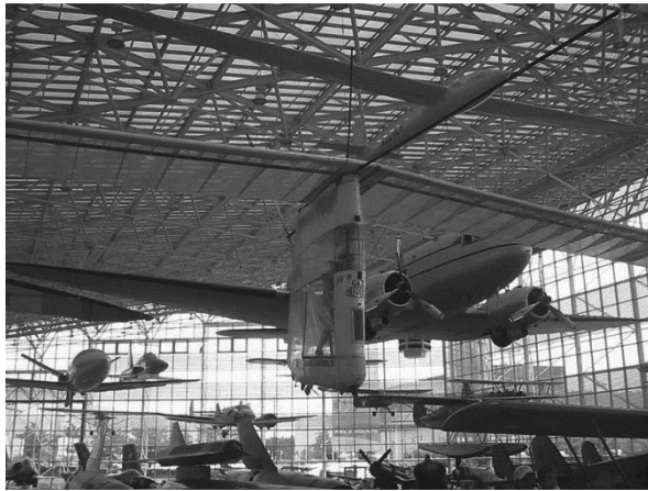
Figure 2.9. The Museum of Flight. The wings of planes are easily recognized as cantilever beams.
