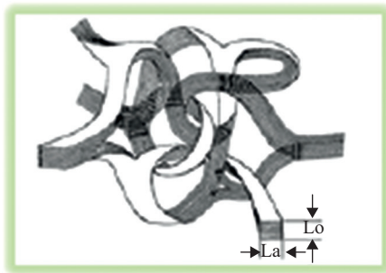
Figure 1.9. Microstructure of glassy carbon proposed by Haris [10], Jenkins and Kawamura [11], and Jenkins [12].
