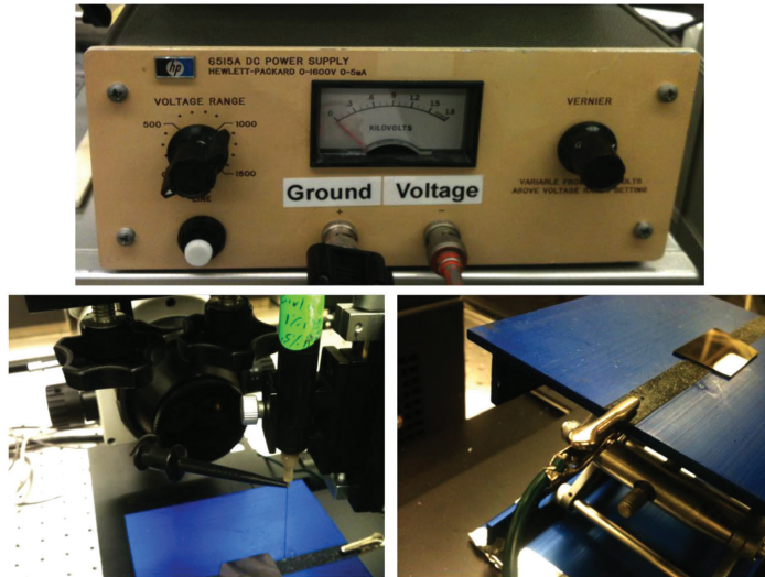
Figure 5.10. Photographs of voltage supply, syringe, and grounded substrate of EMS setup [8].
