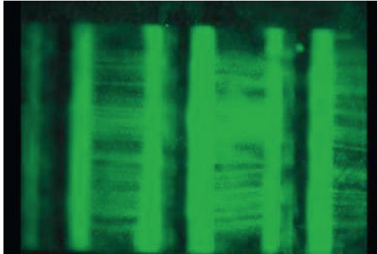
Fluid motion indicated by fluorescent tracer particles and driven by electrical forces over C-MEMS electrodes.
