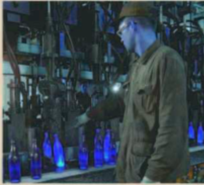
Glass bottles are shaped from molten glass.
