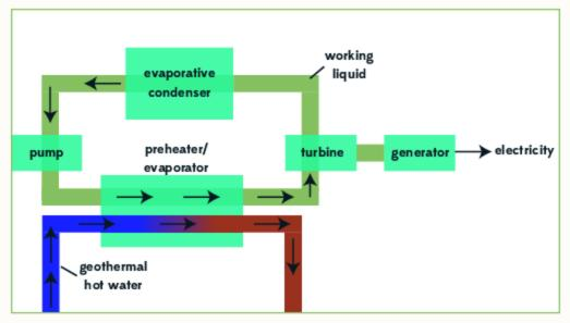
Diagram of a Binary Cycle Geothermal Power Plant
