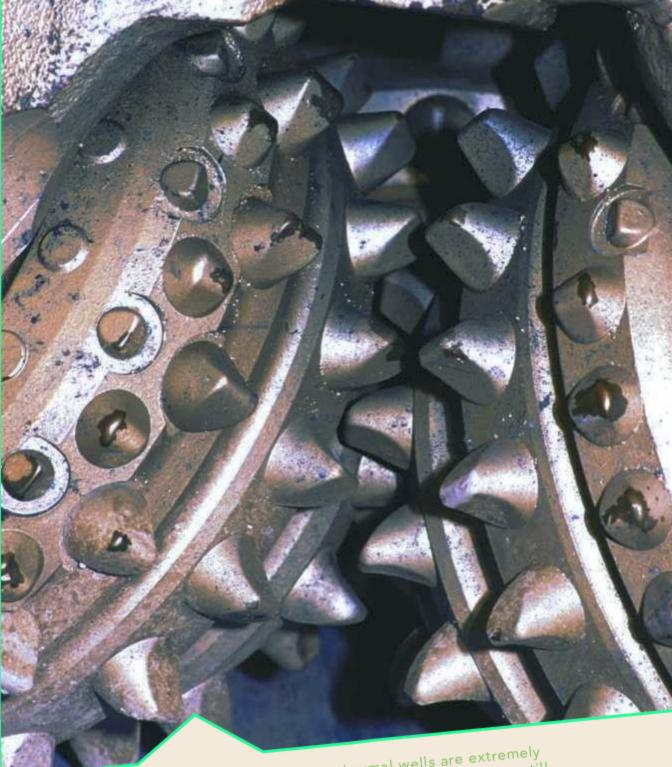
Drill bits used to dig geothermal wells are extremely tough, but the harsh conditions underground can still wear them down.
