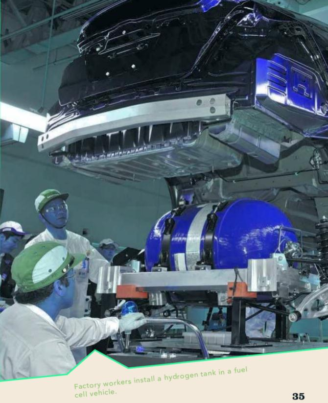
Hydrogen is only a liquid when it is below —423.2 degrees Fahrenheit (–252.9°C). A tank would have to withstand extremely cold temperatures. For compression systems, the material would need to be strong enough to handle extremely high pressures. The tank would also need to resist damage. Most fuel cells need very pure hydrogen. A tank that cracks or flakes would make the gas impure. Scientists are figuring out solutions to these problems.
