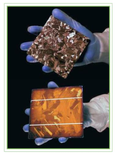
Top, a worker holds a silicon wafer early in the production process. Bottom, a worker holds a photovoltaic cell late in the production process.
