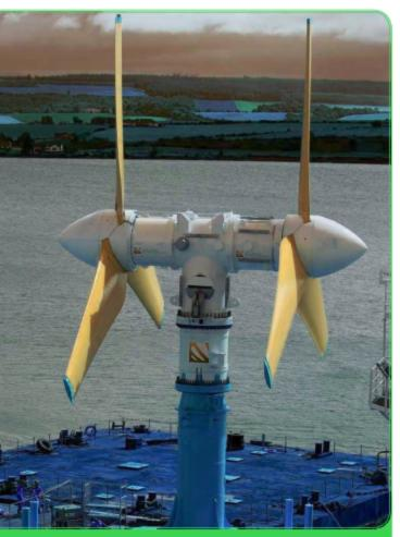
When placed in the water, this large tidal energy turbine will act like an underwater windmill. The moving water, due to the tides, will turn the turbines to make electricity.
