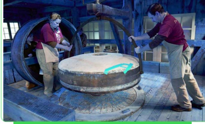
A waterwheel on the outside of a mill can turn a millstone inside the building. This stone, at a museum in Plymouth, Massachusetts, is grinding corn.
