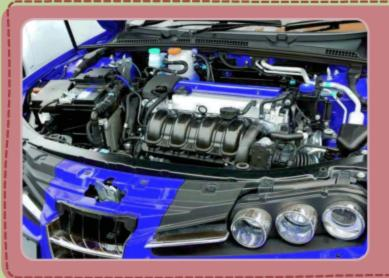
Heat and flames produce a rhythm in something that you know very well—cars. An electrical spark causes gas fumes to **ignite** and expand in cylinders inside the engine. The expanding gas pushes pistons up, and cooling gas lets them come down again. This up-and-down motion is fast and constant, and it provides the "drive" that moves the car.
