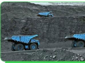
Coal is the most plentiful fossil fuel. After it is dug up, the coal is loaded into trucks that take it to be crushed. That makes it easier to ship and burn.
