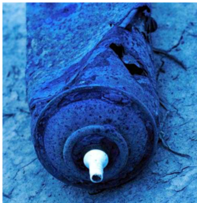
This steel container is rusting. A chemical reaction occurs when the iron from the can meets the oxygen in the air.
