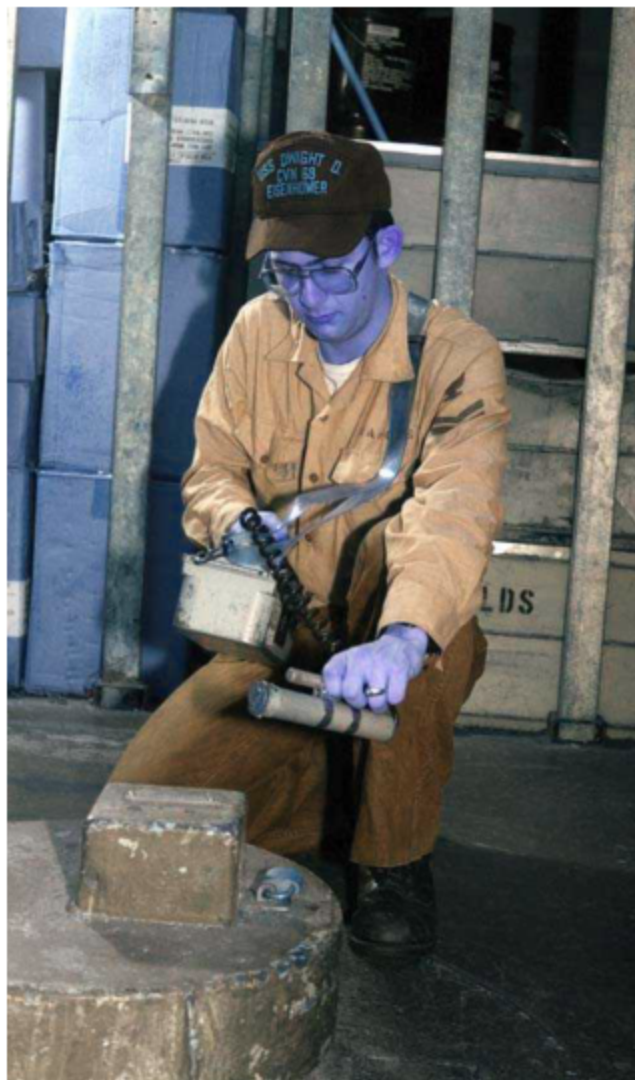
This man uses a Geiger counter to determine the presence of radioactive materials.
