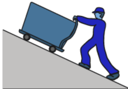
The first ramp is longer, but its slope is gentler. The second ramp is shorter, but its slope is steep. Both jobs take the same amount of work to complete.
