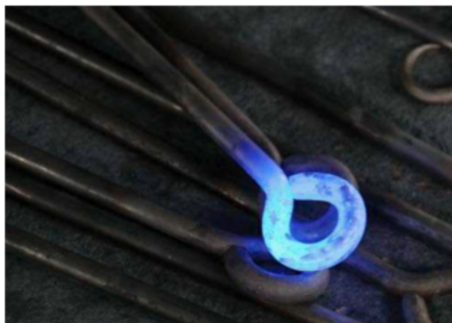
A red-hot iron rod will transfer heat to the surrounding environment through radiation.
