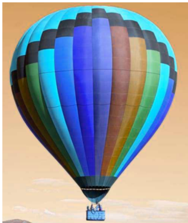
Hot air balloonists control their height by adding hot air to the balloon, or by releasing it.
