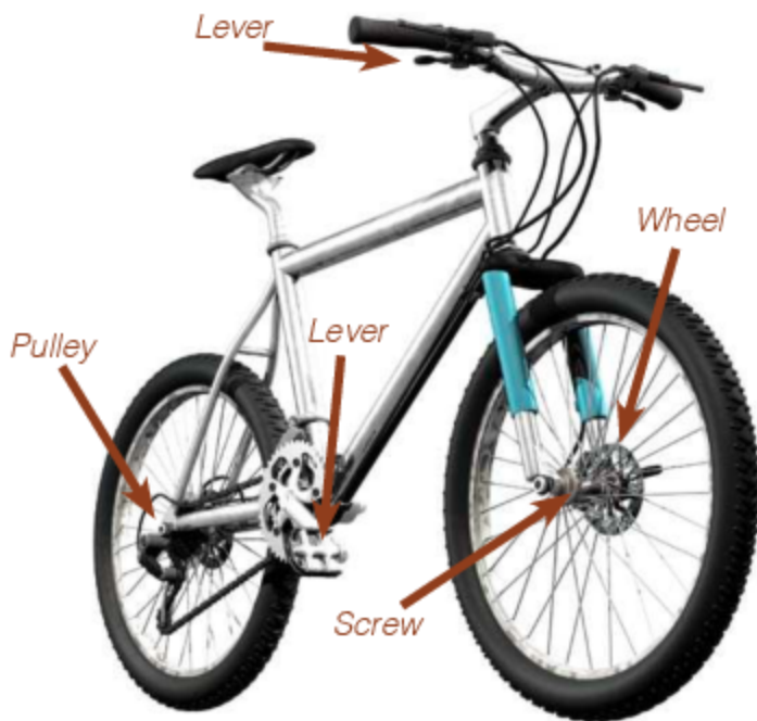
The bicycle is a complex machine that contains many simple machines.
