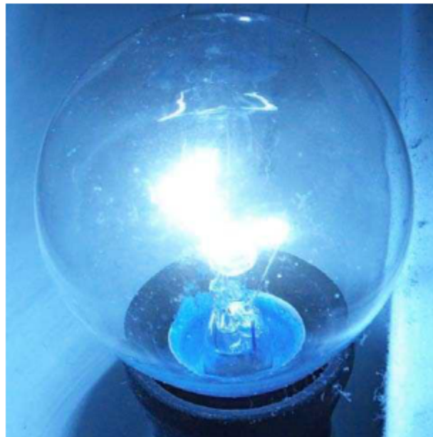
An electric current passes through the filament in this light bulb and causes it to glow.
