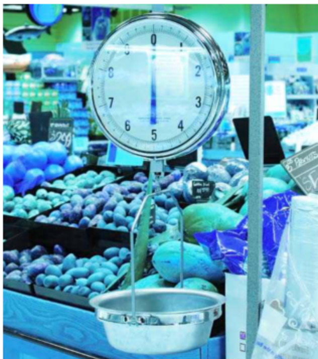
This scale is used to measure the weight of fruits and vegetables in a grocery store.
