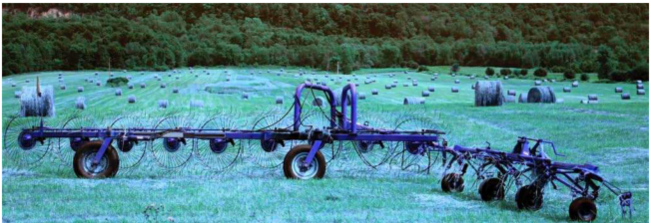
Wheel rakes attach to tractors and sweep cut grain crops into piles. Often farmers use other equipment to make the piles into bails.
