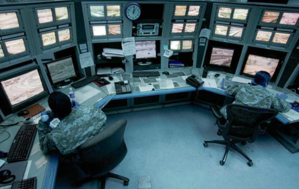
In 2007, at a Border Patrol processing center in El Paso, Texas, members of the Texas National Guard monitor dozens of cameras for illegal border crossings. Electronic sensors, authorized the previous year, activate cameras that capture movements along the border.
